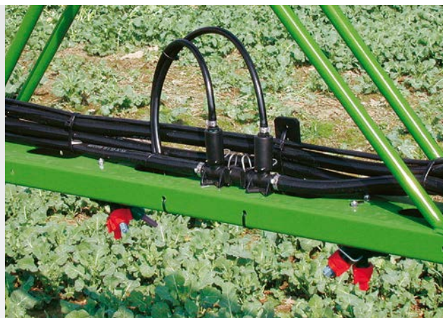
DUS pressure recirculation system
