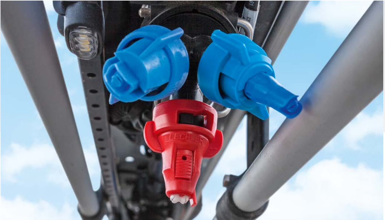
AmaSwitch triple nozzle body with LED individual nozzle lighting
