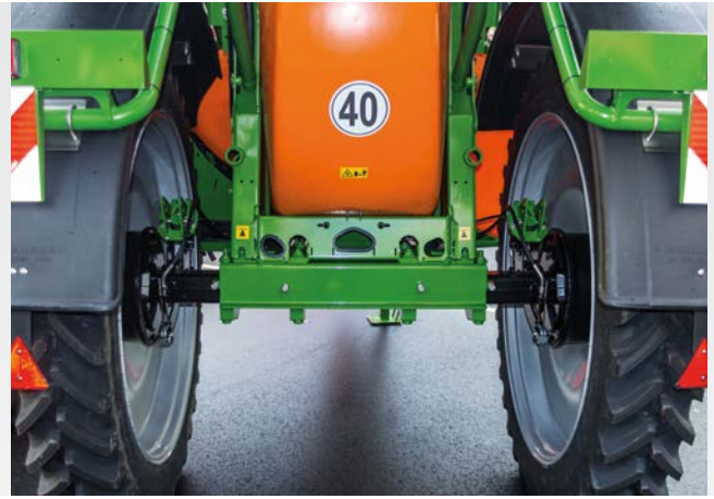
Adjustable axle with step-less track width adjustment from 1.50 m to 2.25 m for the UX 4201
