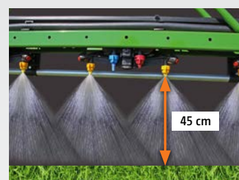
80° nozzles: 25 cm nozzle spacing
