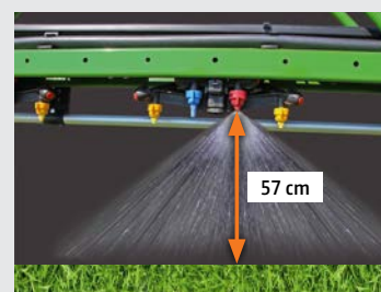
110° nozzles: 50 cm nozzle spacing
