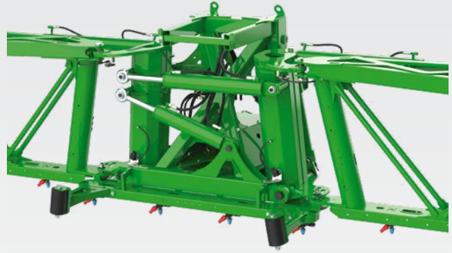
Swing compensation system for Super-L3 booms from 39 m
