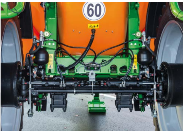
Hydro-pneumatic axle suspension with AutoTrail axle steering for the UX 4201 and UX 5201
