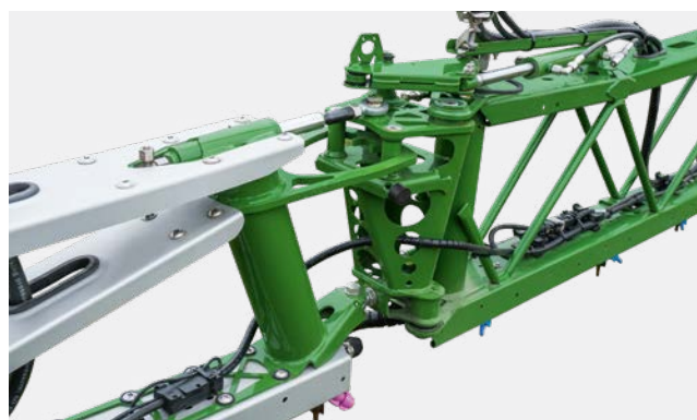
The hydraulically pressurised break back system on the boom end (which works just like the saloon door principle) can cope with obstacles from the back, front or from the top and ensures a reliable return to the working position and a long service life.
