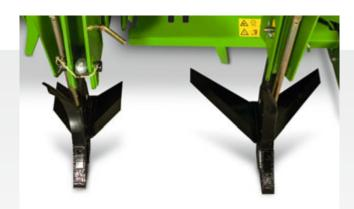
30 cm wing shares are used as standard. A wider loosening 60 cm wing share and a side plate extension are available as an option.
