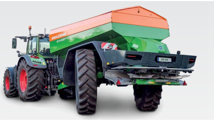
Steering axle with a steering angle up to 28°
