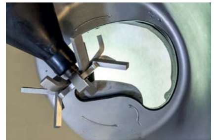
Stage 3: hopper shutter wide open
