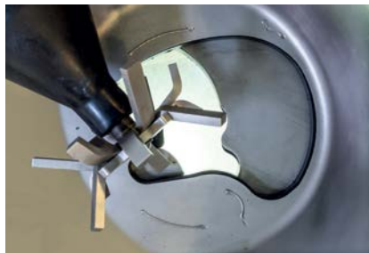
Stage 2: hopper shutter half open
