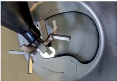
Stage 1: hopper shutter slightly open
