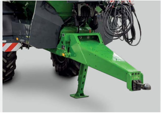
✔ Hitch coupling with K80 ball coupling
