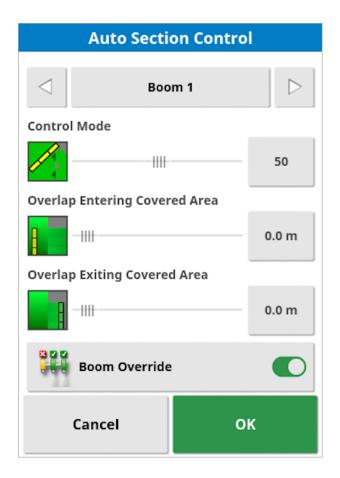
Boom override turns off section control for this boom. Select the required boom and press **Boom Override**. At least one boom must be turned on. Use **ASC on/off** on the mini-view to turn off all booms.
