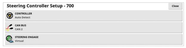
Controller: Note: It is important to select the specific steering controller, if it is listed, so that auto steering settings match the vehicle profile. Note that if the steering controller is changed later, it may be necessary to return to the vehicle geometry to confirm the dimensions (refresh them). Note that Auto Detect does not automatically detect the controller options that are available in the list, so the specific controller must be selected if it is an available option.
