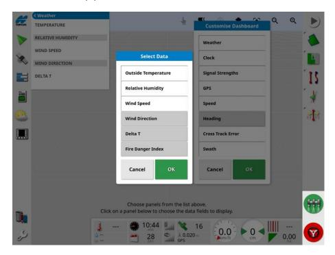
Once connected, both a mini-view and the dashboard can display temperature, relative humidity, wind speed, wind direction and Delta T.
