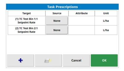
Target: The tank or bin that is being controlled. Select \* to add another target.
