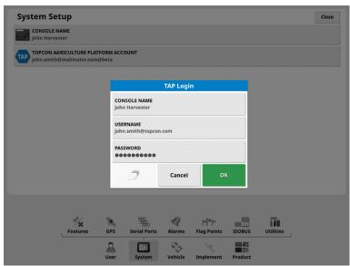
Once the display is logged into TAP, it will establish communication whenever a TAP operation is required and internet is available.
