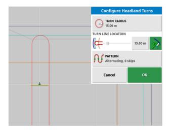
A larger turn radius provides a keyhole shaped curve.
