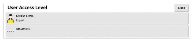
The Access Level may be set at Easy, Standard or Expert. A password may be set for the Standard and Expert levels to prevent inexperienced users from accessing higher levels.
