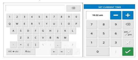
Letter and number keypads are used to enter alphanumeric characters or numeric characters. Entries must be confirmed.
