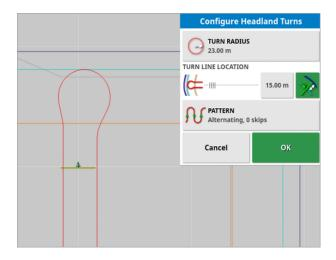
**Note**: To ensure that the implement is correctly on the line when exiting the headland (returning into the field) the shape of the curve may be such that the vehicle's initial movement is away from the next line, or the approach to the next line may have the vehicle overshoot the line. This is intentional and helps to ensure that the implement enters correctly without leaving gaps. See the following image.
