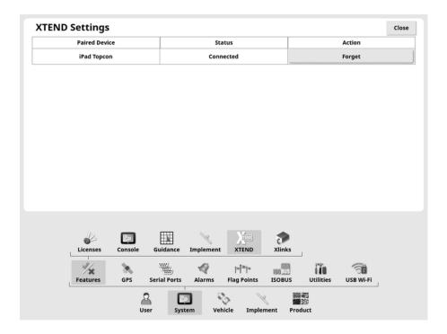
The **Forget** option prevents an external device from reconnecting to this display via XTEND, unless the display operator confirms the connection.
