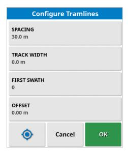
• Spacing: The distance between the centers of the tramline passes. Usually this will be the width of the sprayer.
