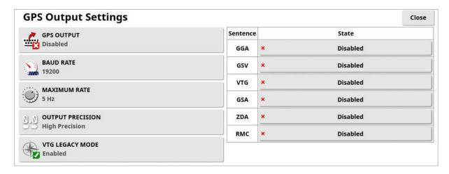
VTG legacy mode: Supports VTG data output for NMEA standards below V4.00. Outputs VTG strings compatible with NMEA V3 and below.
