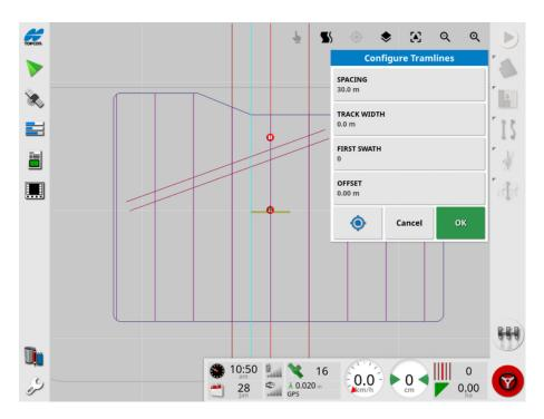
The tramlines are shown in purple and an alarm is shown to advise a user they are on a tramline pass. The tramline pass alarm displays if the vehicle is driving across a tramline.
