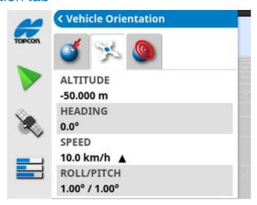
This shows altitude, heading (degrees), actual speed of the vehicle and roll/pitch (degrees). Roll is the left/right tipping of the vehicle. Pitch is the forward/back tipping of the vehicle.
