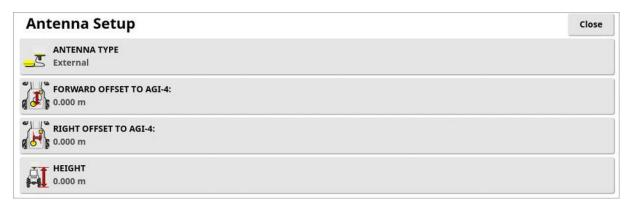
If **External** is selected, the measurements for the location of this antenna must be entered:
