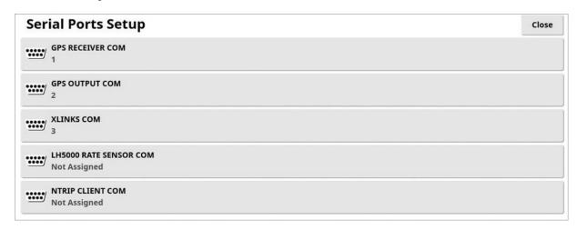
2. Select the required function and from the selection list, select the display serial port to which the device is connected.
