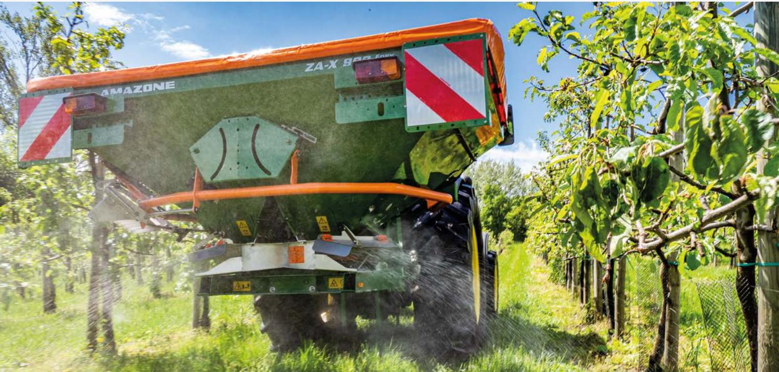
ZA-X 903 Easy with row spreading attachment in an orchard
