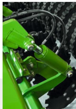
Hydraulic depth adjustment with large scale
