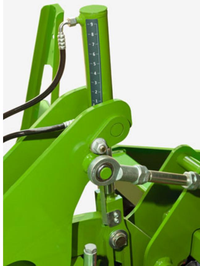
KX/KG hydraulic depth adjustment
