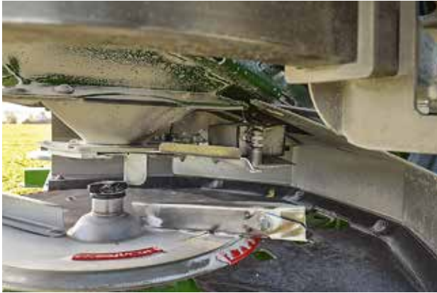
△ The spreading width is changed by adjusting the spreading vanes. The rate is controlled by actuators. Angle sensors measure the aperture.
