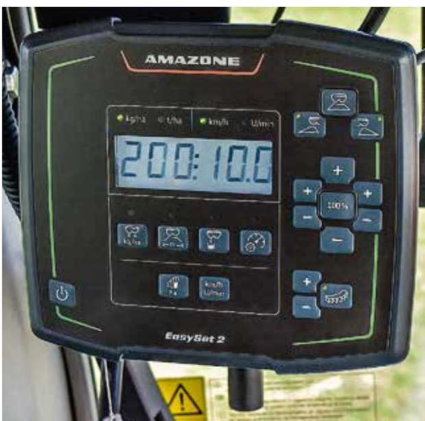
◁ An LED light down in the right corner on the EasySet 2 unit indicates the boundary screen is in position.
