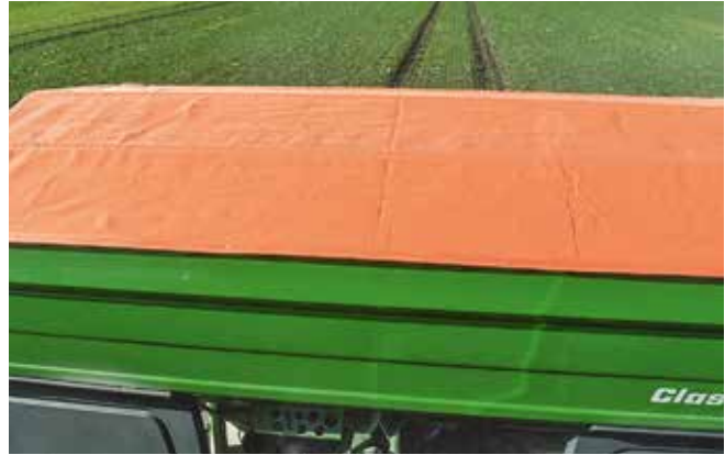
△ Lacking an inspection window, the hopper doesn't allow operators to check the filling level from the seat.
