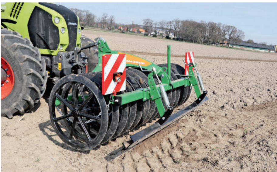
Nautilus is a steered front packer with 900mm cast rings which gives excellent consolidation.
