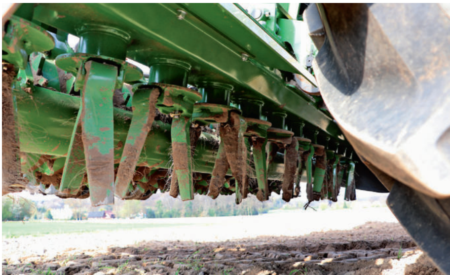
KE 3002 standout features are small rotor heads and inclined tines. The machine handles more tractor power although it's lighter in weight.
