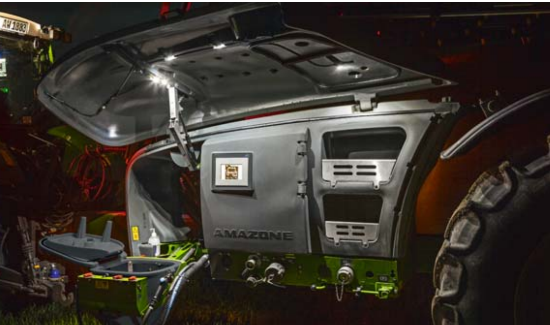
SmartCenter with Comfort-Pack plus and LED lighting, safely protected under the cover
