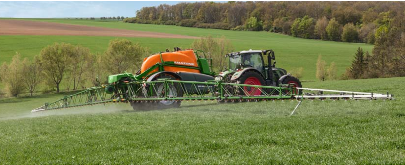
ContourControl with negative boom angling
