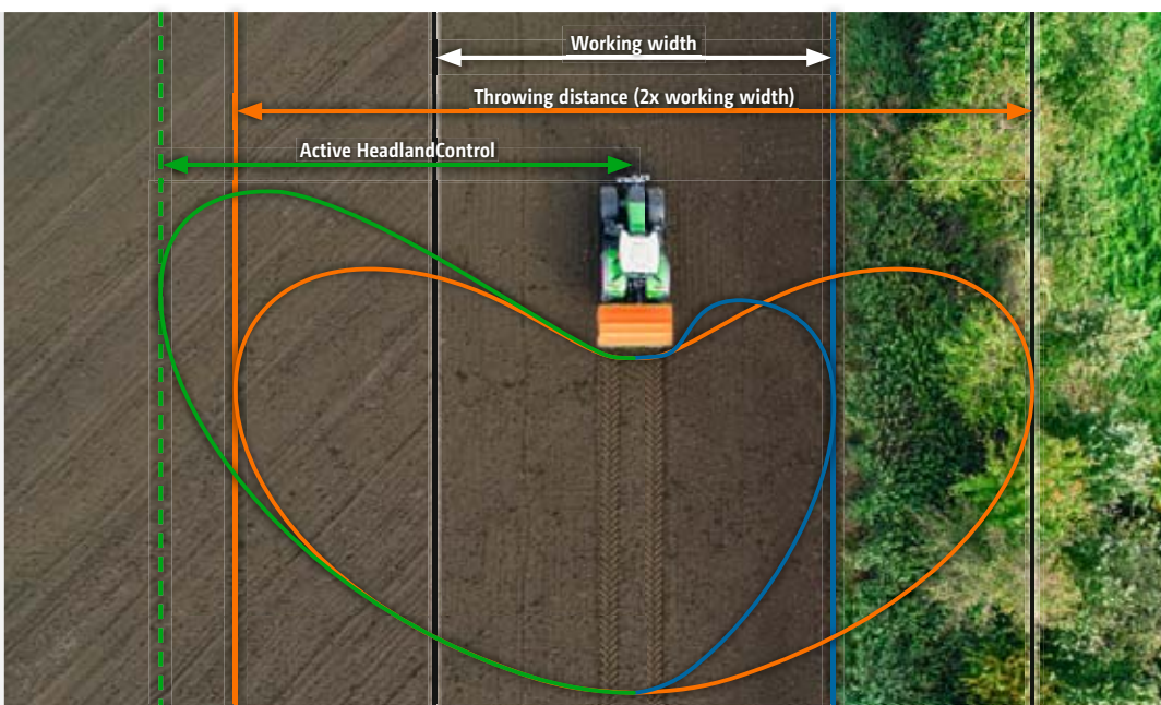
HeadlandControl – optimum lateral distribution on the headland
