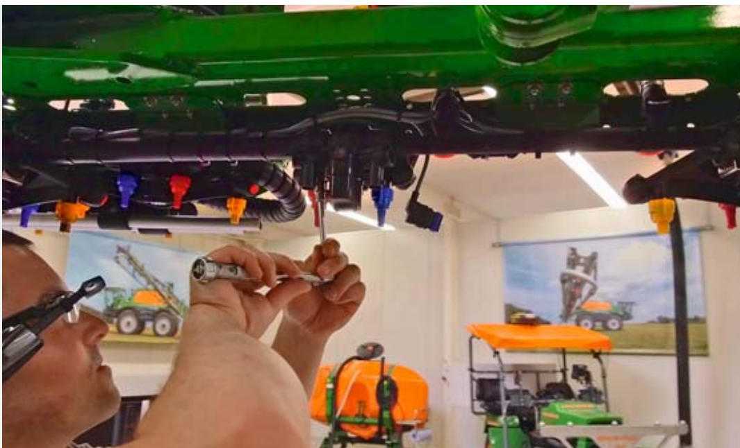
Service technician carrying out a SmartInstruction on the AmaSelect nozzle body
