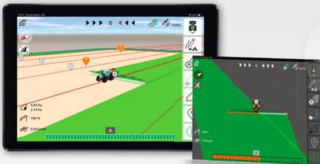
Map view with AmaTron Twin – Clear display of the machine and its part-width sections, as well as buttons on the right-hand side of the tablet display
