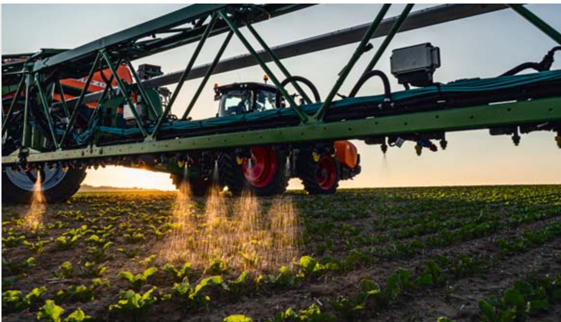
Spot application via the spot nozzle bodies
