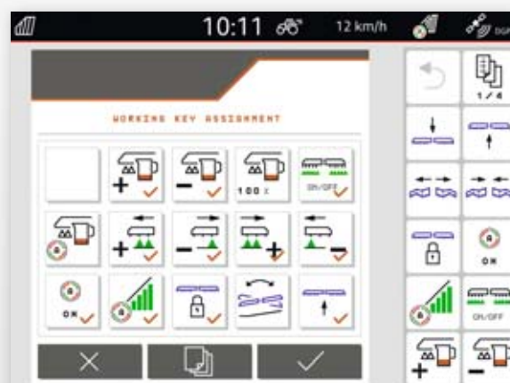
The operator can individually assign functions to each button
