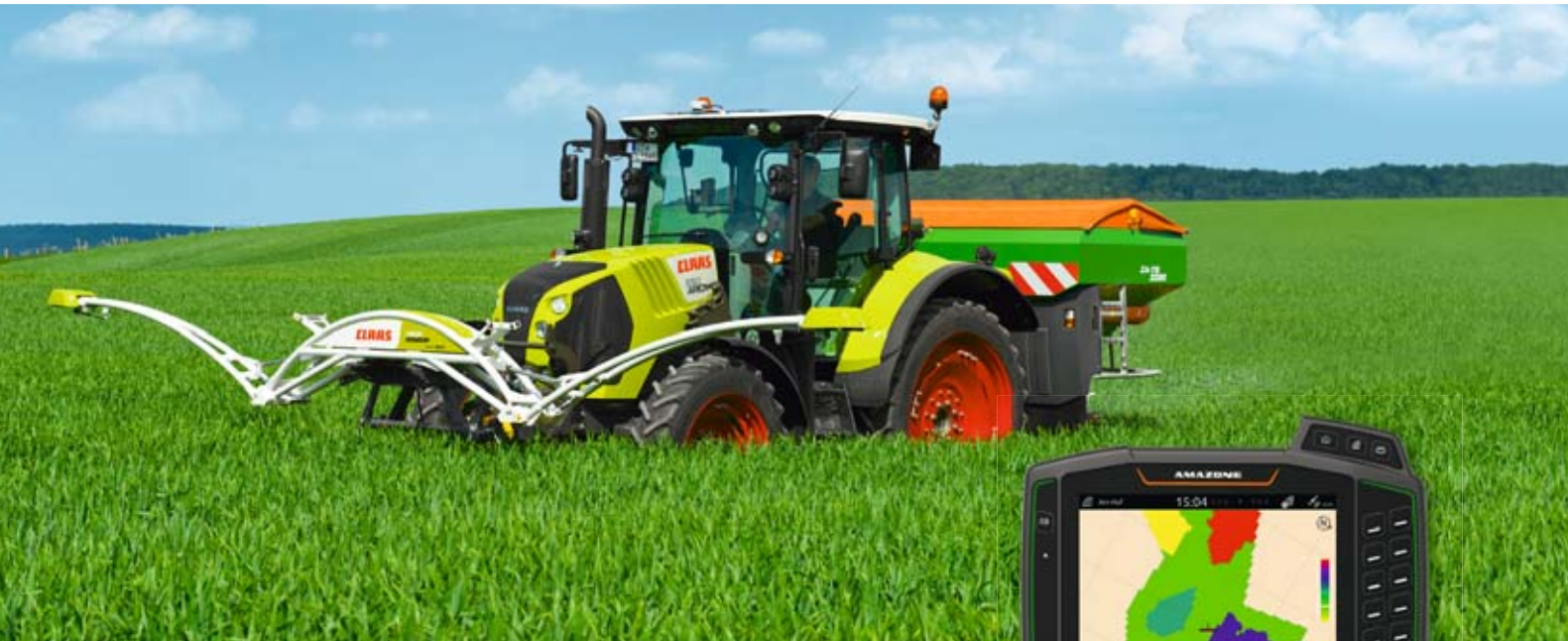
Part-area, site-specific fertilisation with N-sensor
