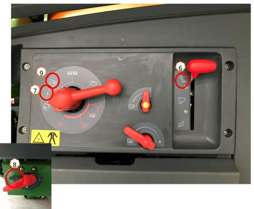
After the sprayer has been filled and the crop protection products have been flushing in, the pressure tap must be switched to "Spraying" (1).
