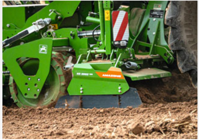
KE 3002-190 Rotamix with DirectDrive gearbox
