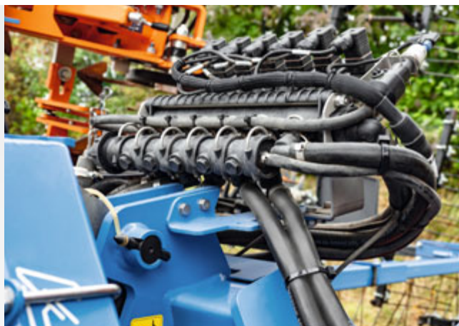
Part-width valve chest on the SCHMOTZER Ventera 2K hoe
