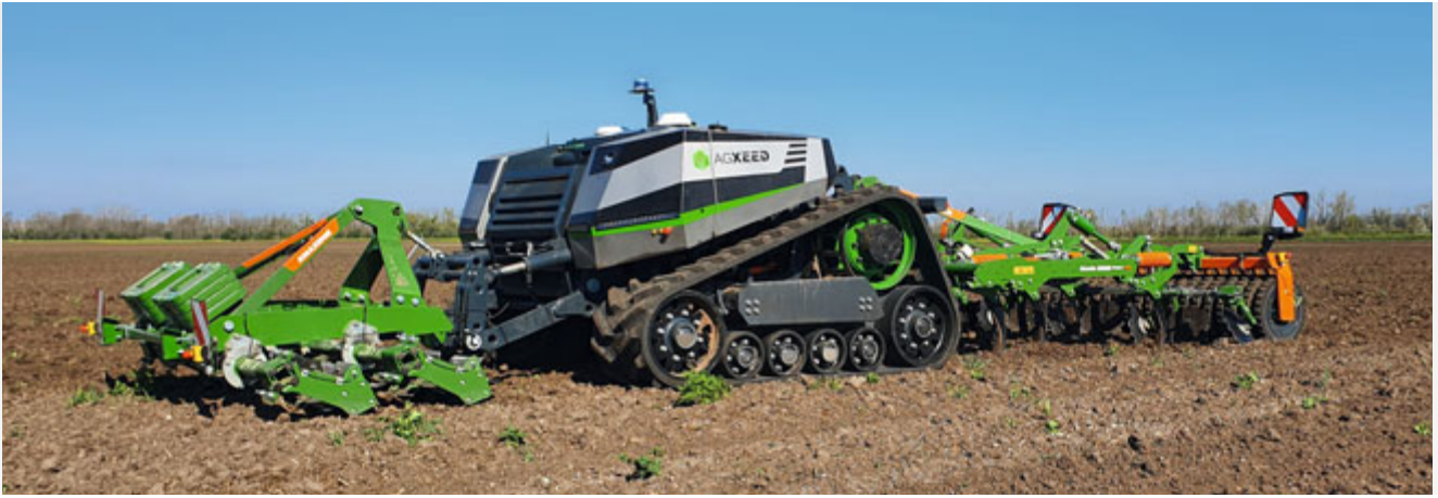
AgXeed AgBot with tracked crawler chassis and AMAZONE Cenio 3000 Super mounted cultivator and front-mounted double knife roller
