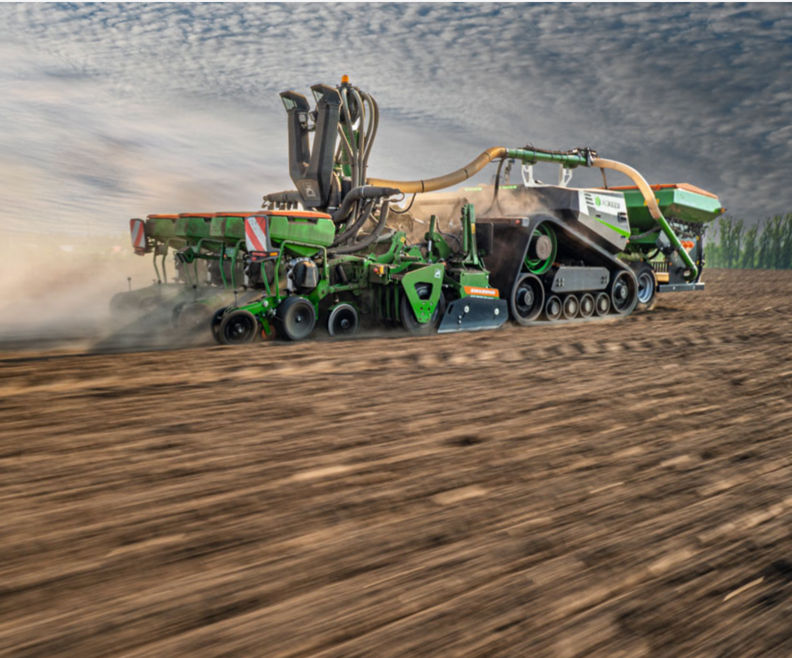
AgXeed AgBot tracked crawler chassis and AMAZONE Precea 3000-FCC precision air seeder with FTender 1600 front mounted hopper
