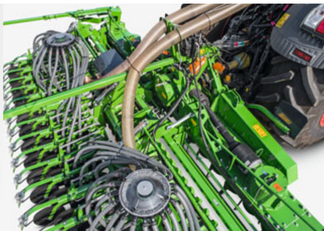
Double transfer pipes with twin distribution heads on the Avant 6002-2
