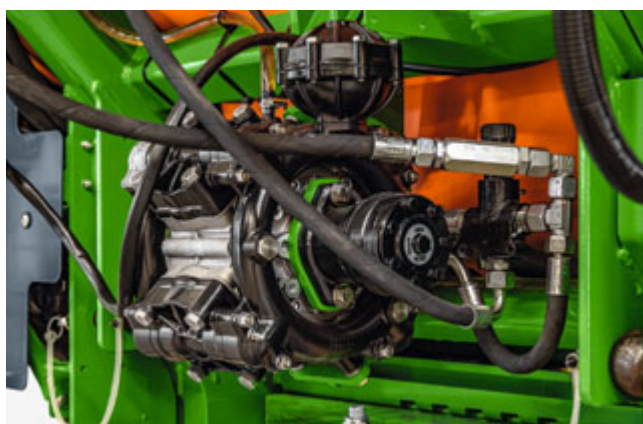
Hydraulic pump drive, with a safety valve to prevent over-reving and incorrect hose connection to the tractor
