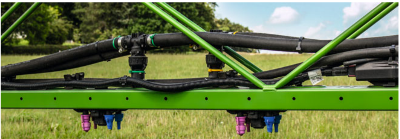
The boom has two separate supply lines, yellow and green, which are switched remotely
