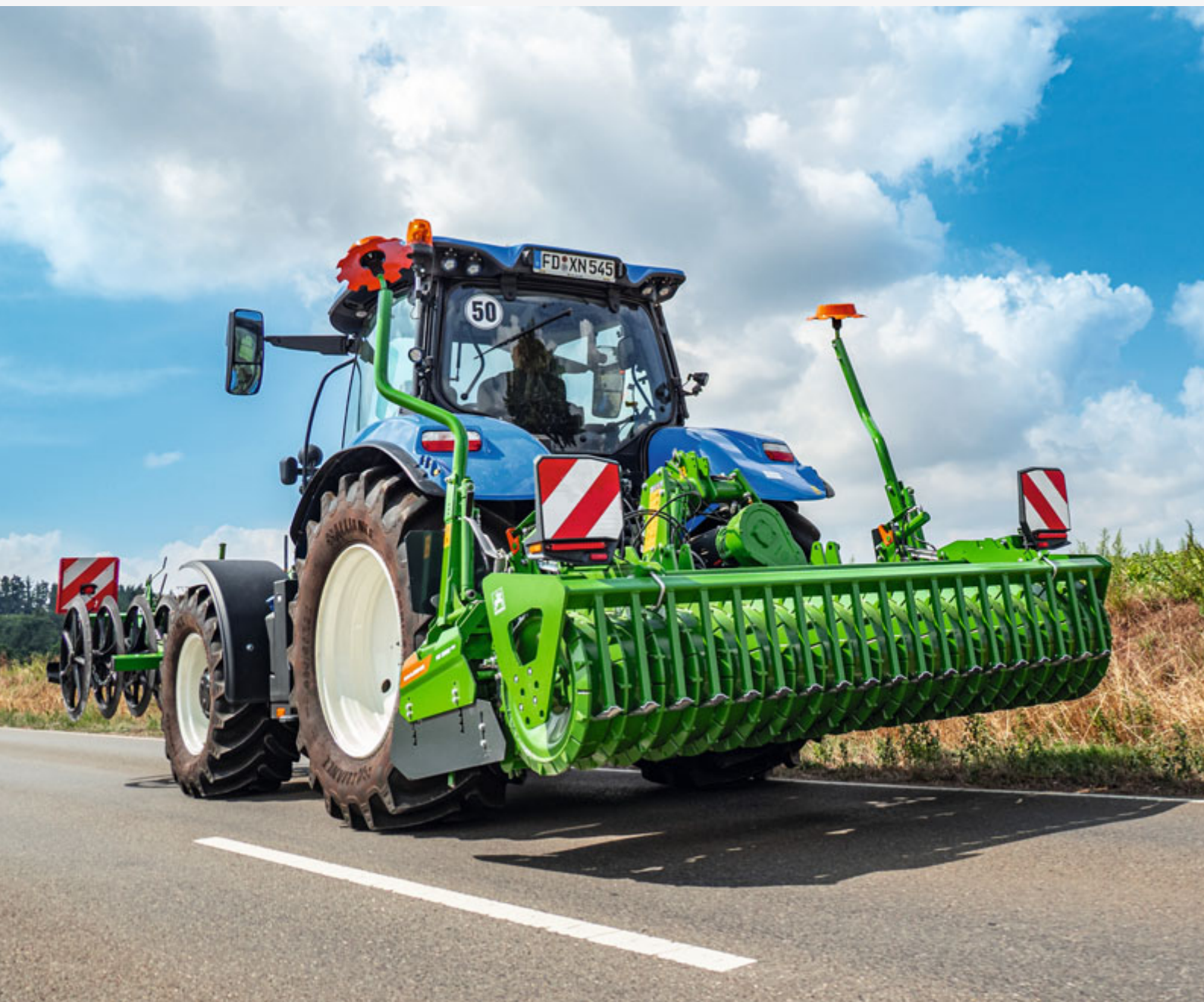
The rotary harrow can be equipped with marker boards and road lights for solo operation
