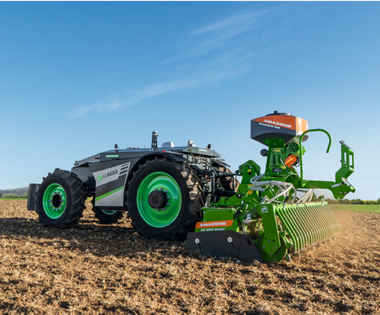
4-Wheel AgXeed AgBot and AMAZONE KE 3001 Super rotary harrow with GreenDrill harrow-mounted catch crop seeder box
