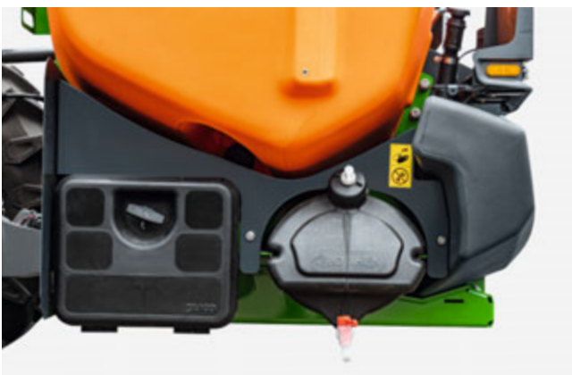
Lockable storage compartment and hand wash tank with integrated soap dispenser on the right-hand side of the machine
