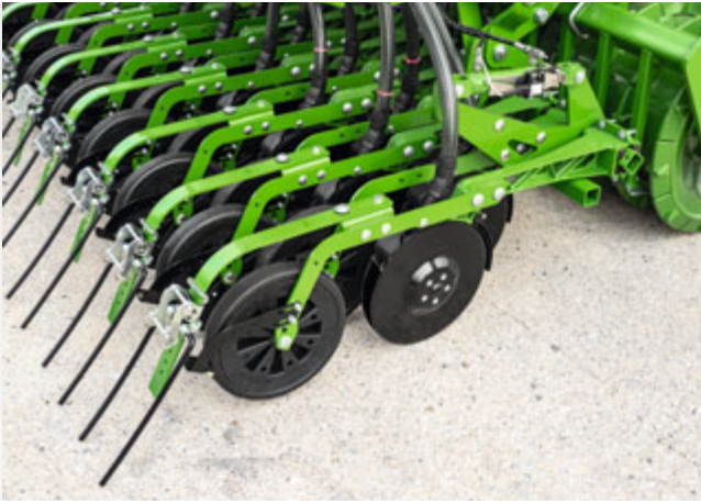
TwinTeC Special double disc coulters with single-arm steering
