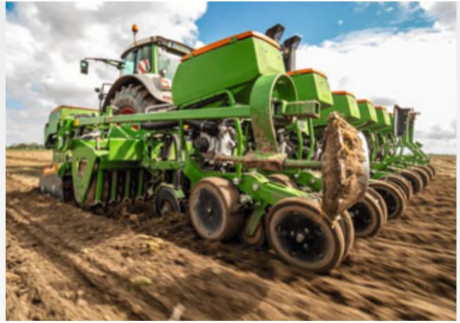
Precea singling units mounted on the KG 6002-2 Super ensure precise placement of the seed.
