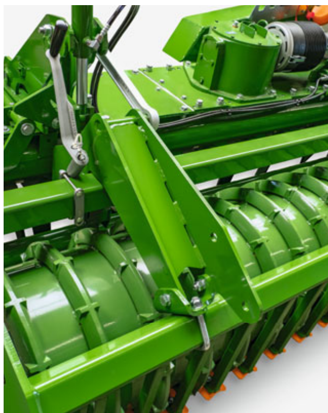
Coupling point for a quick change between Precea seeding units and the Avant 02 seed rail
