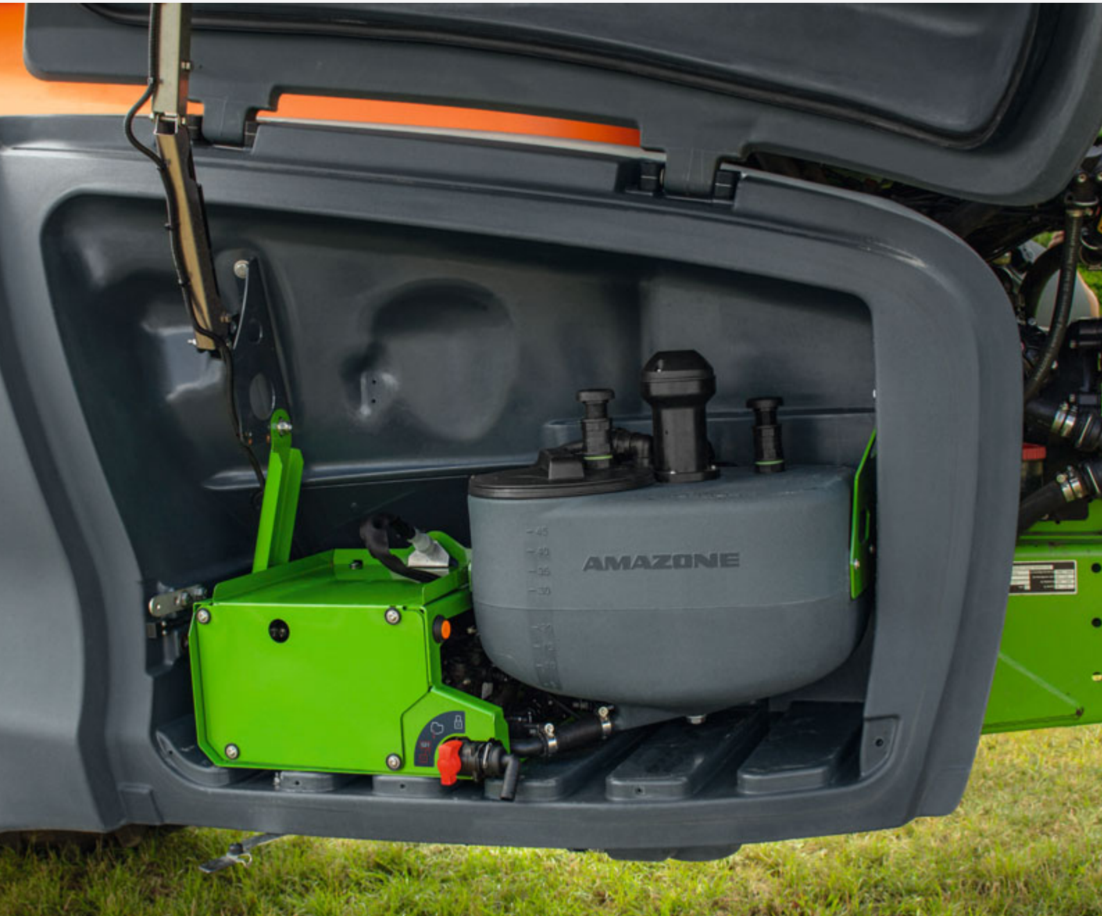
DirectInject equipment with 50 l tank and pump unit in the storage compartment of the UX 01 Super
