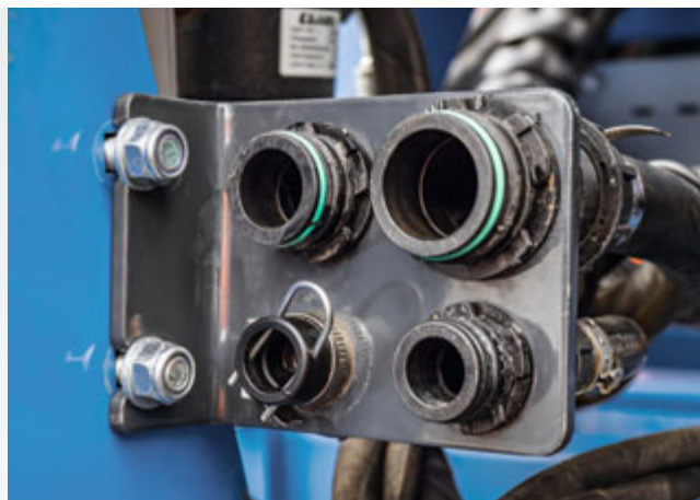
Interface between the FT-P 1502 front tank and part-width valve chest on the attached implement
