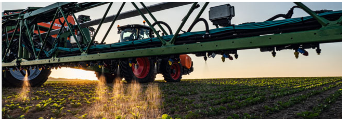
Spot application via the spot nozzle bodies
