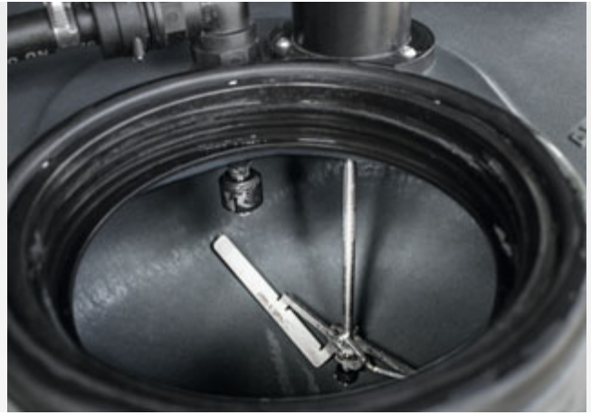
Mechanical agitator and cleaning nozzle in the DirectInject tank
