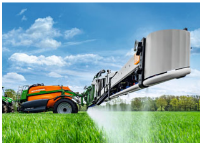
UX 7601 Super with a one-piece chassis without a separate drawbar for an extremely low centre of gravity
