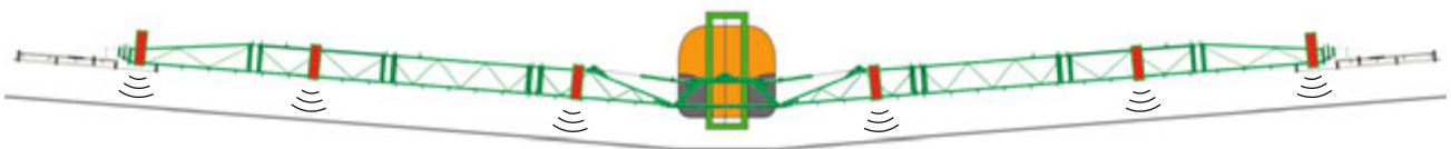
Simultaneous positive angling (Flex fold)
