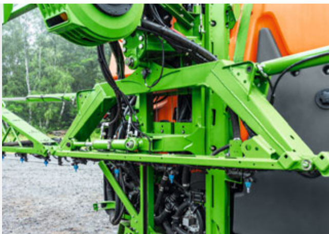
Fully automatic, active ContourControl boom guidance
