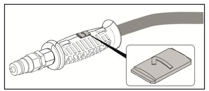
Films are stuck on the implement for the markings that illustrate the respective hydraulic function.
