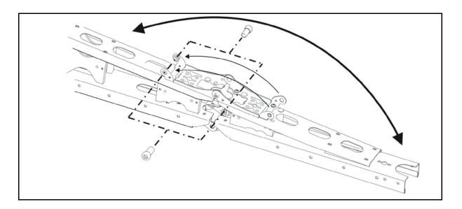
2 bolts lock the folded and unfolded outer element in its respective end positions.
