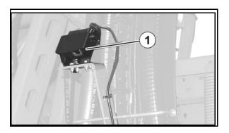
(1) Camera on the front tank for manoeuvring safely.
