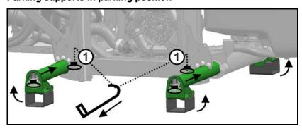
Hook the pulling rod on the lug (1) and pull to move the parking support into transport position.
