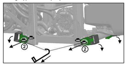
Hook the pulling rod on the lug (2) and pull to move the parking support into parking position.
