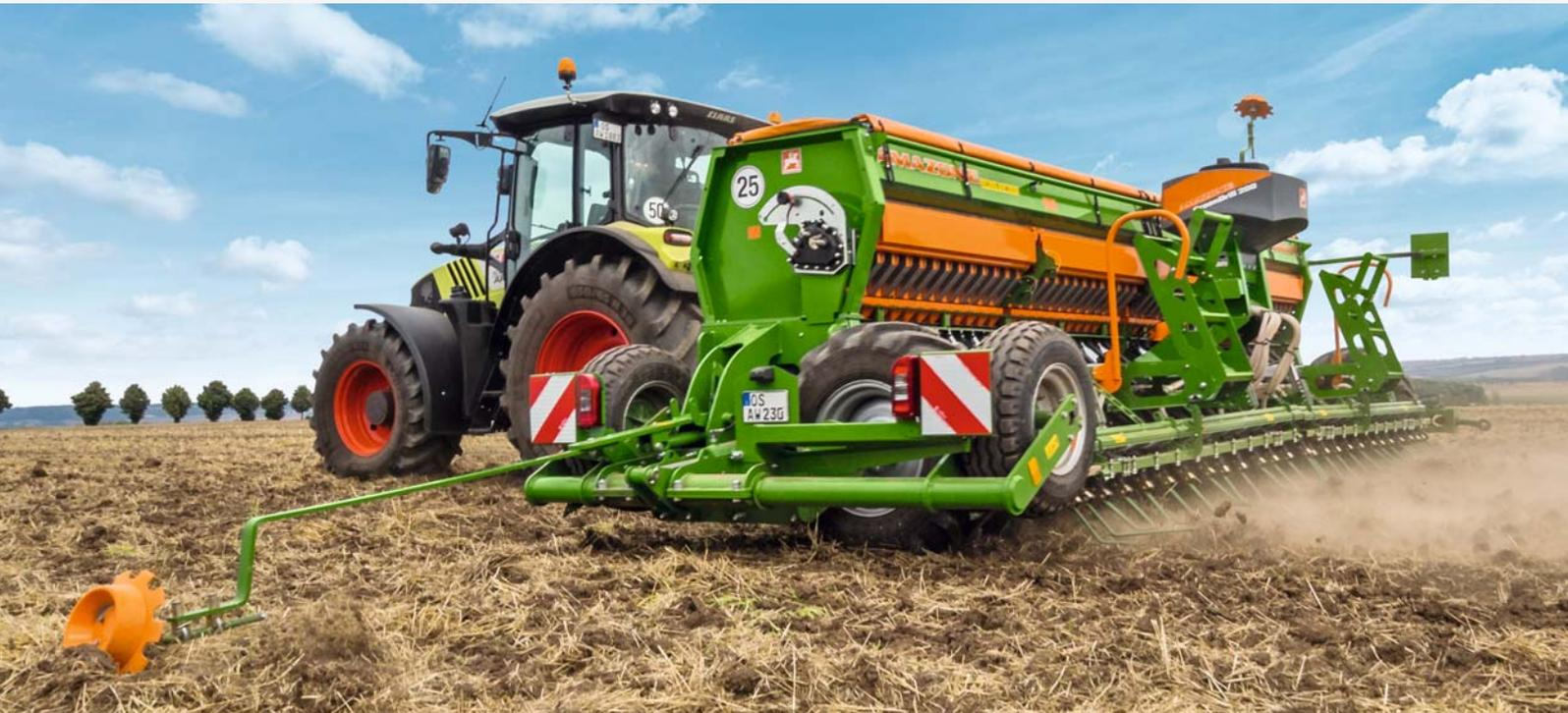
The D9 "Combi" with a working width of 6 m has established itself successfully in the Russian market and is perfectly suited for mounting onto smaller tractors with little lifting power.
