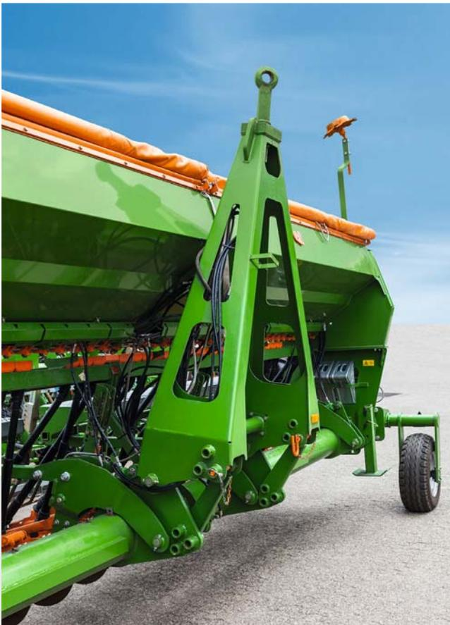
Hydraulically-folding transport drawbar
