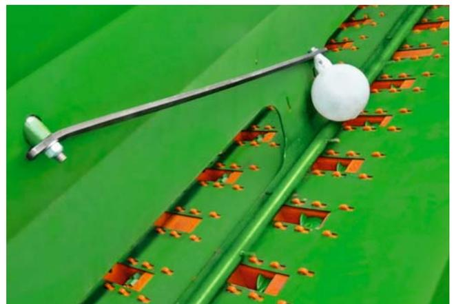
Via the removal of the partitions and closing off the fertiliser metering system, the complete hopper volume can be utilised for seed.
