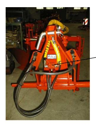
Valve for steering and track width adjustment - furrow width, furrow 1 (lever at zero)
