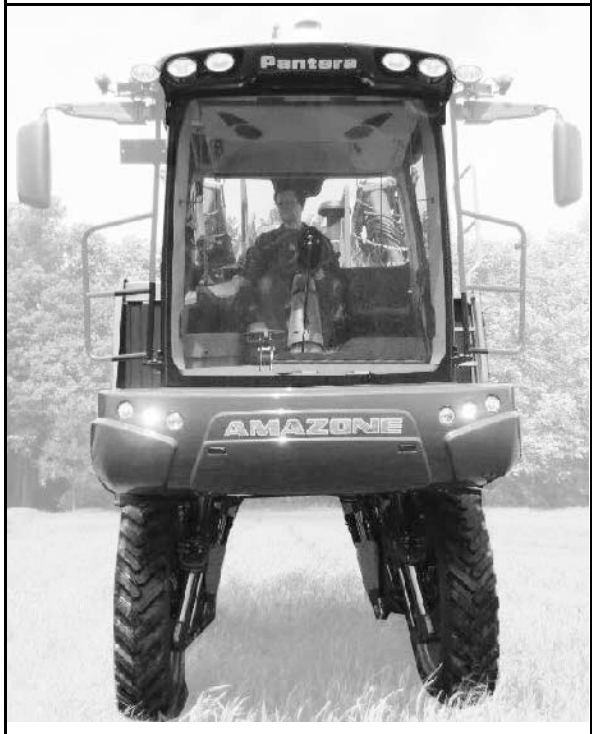
Machine raised (only for driving on the field)
