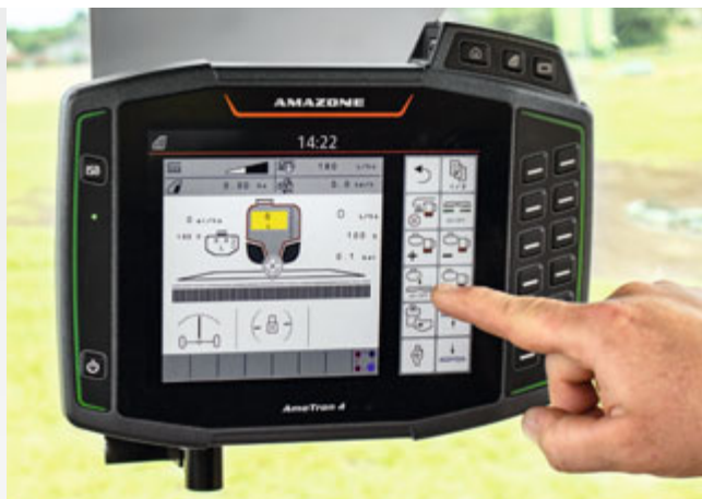
Activation of DirectInject in the AmaTron 4 terminal
