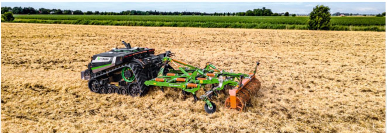
The AgBot from AgXeed with an output capacity of 156 hp and a conventional 3-point linkage
