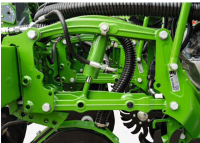
The coulters pressure is adjusted automatically via the hydraulic cylinder on the Precea Super
