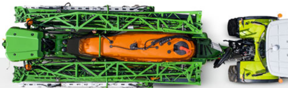
42 m working width compactly folded for safe road transport
