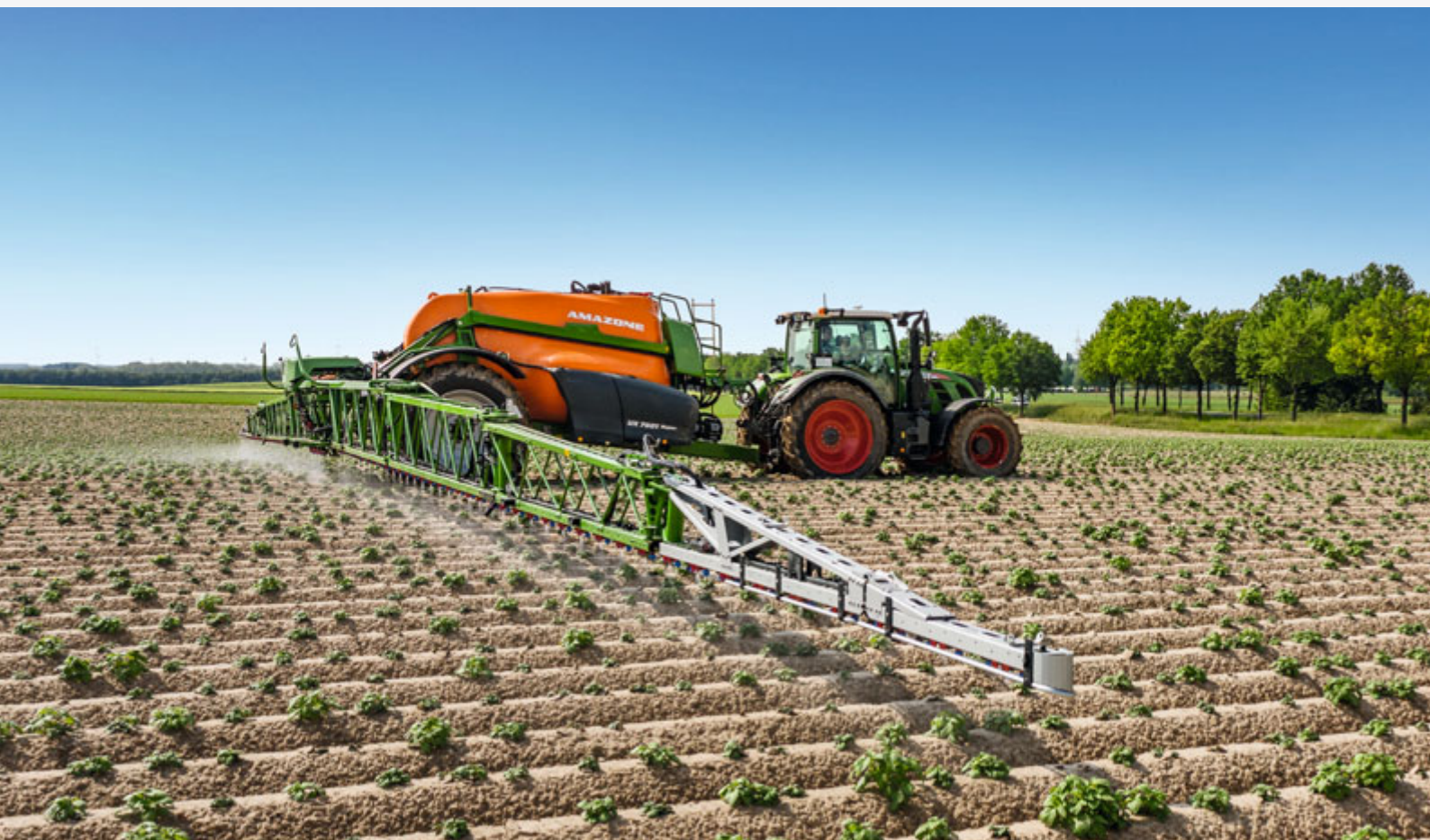
UX 7601 Super with 42 m Super-L3 boom: Precise boom guidance thanks to ContourControl and SwingStop
