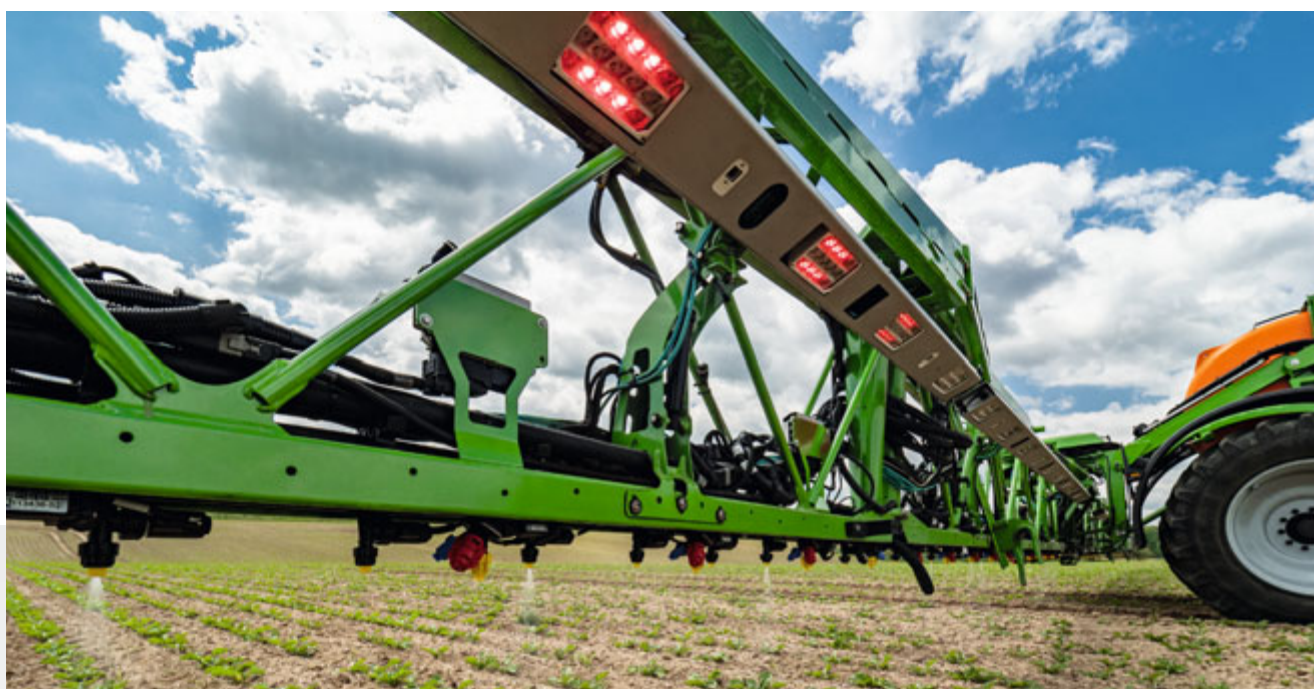
Active light source for accurate weed detection by day and night
