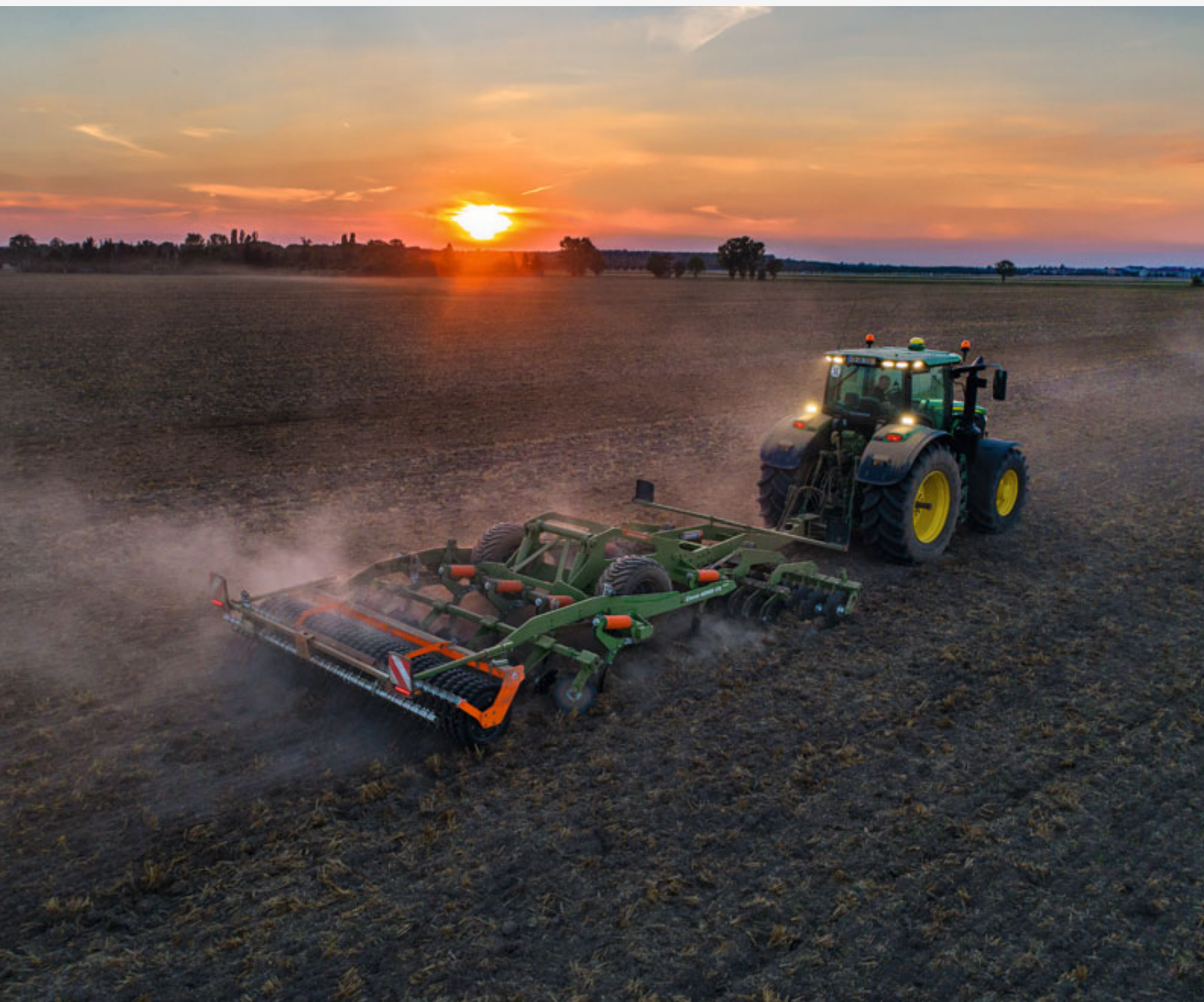
Ceus 4000-TX disc & tine combination cultivator for intensive mixing and deep soil loosening
