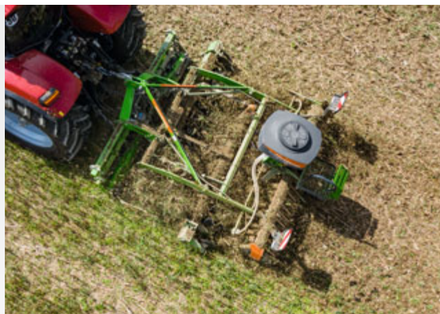
The X-Cutter disc ensures a particularly high proportion of fine soil. This provides the optimum germination conditions when used for the simultaneous broadcasting of catch crops.
