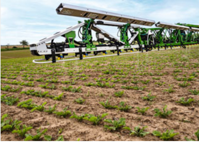
Boom end with integrated break back protection
