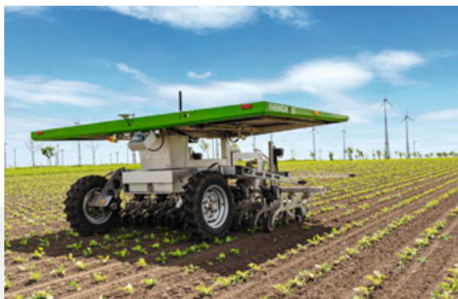
The FarmDroid FD20 robot is equipped with a GPS seeding system, a hoe and the innovative AMAZONE precision spraying system for spot applications
