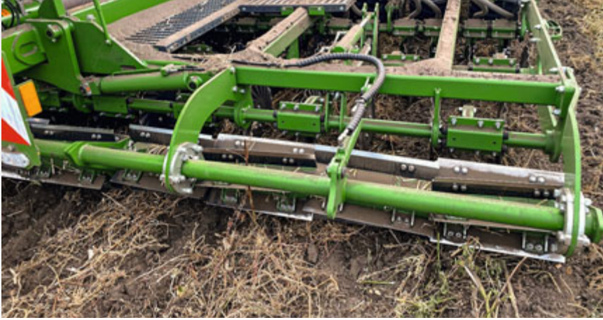
The knife roller as an aggressive front tool for the Cirrus 6003-2
