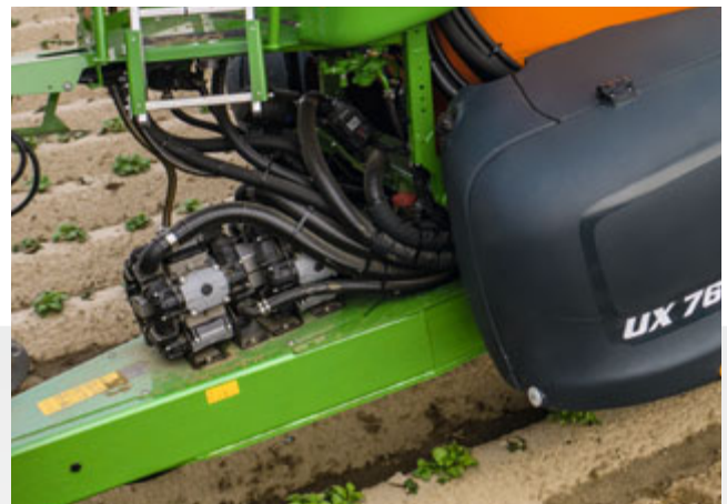
Newly developed piston diaphragm pumps with hydraulic drive
