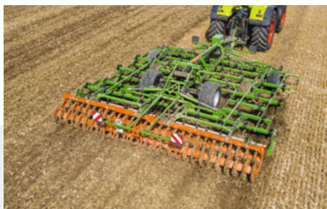
Full surface movement and intensive incorporation of organic matter thanks to the 6-stagger layout
