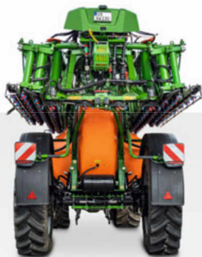
42 m working width compactly folded for safe road transport
