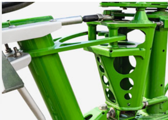
Hydraulic pre-tensioning of the boom end
