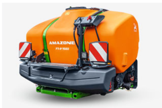
Folding platform with access step for safe introduction of supplementary products
