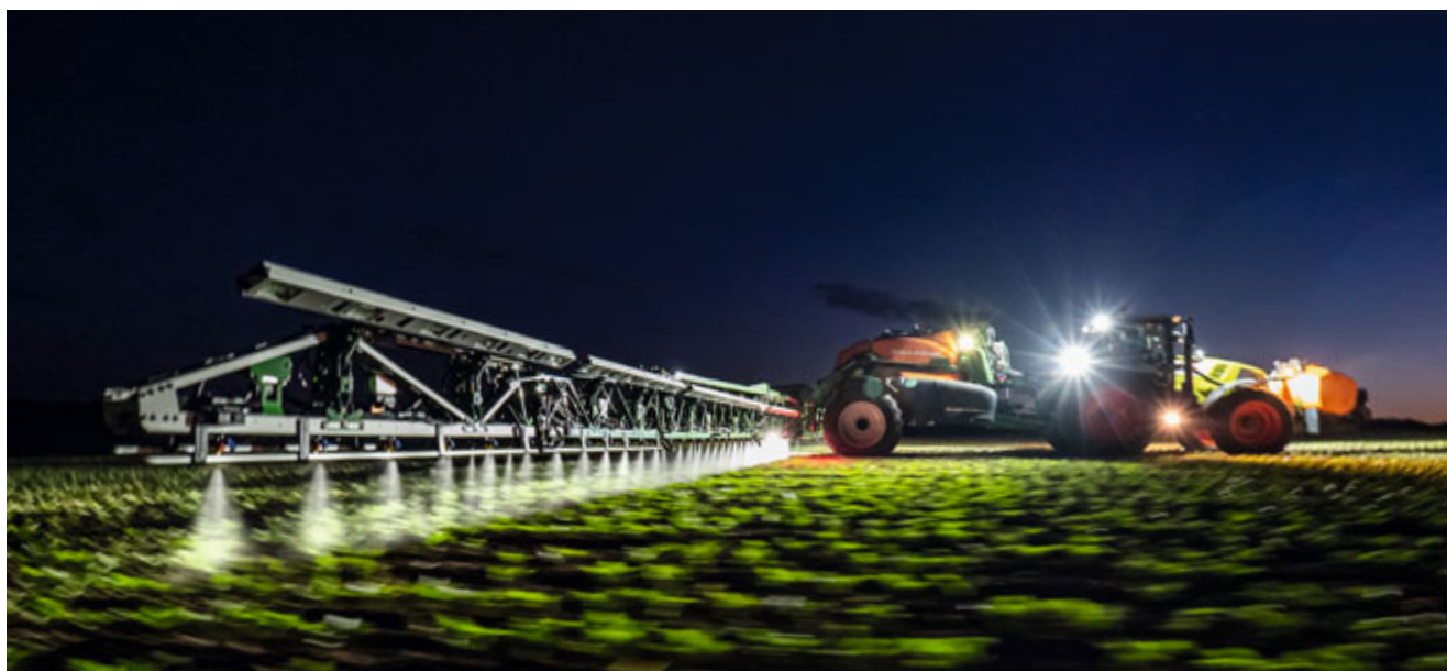
Combination of full-surface application and spot application at night
