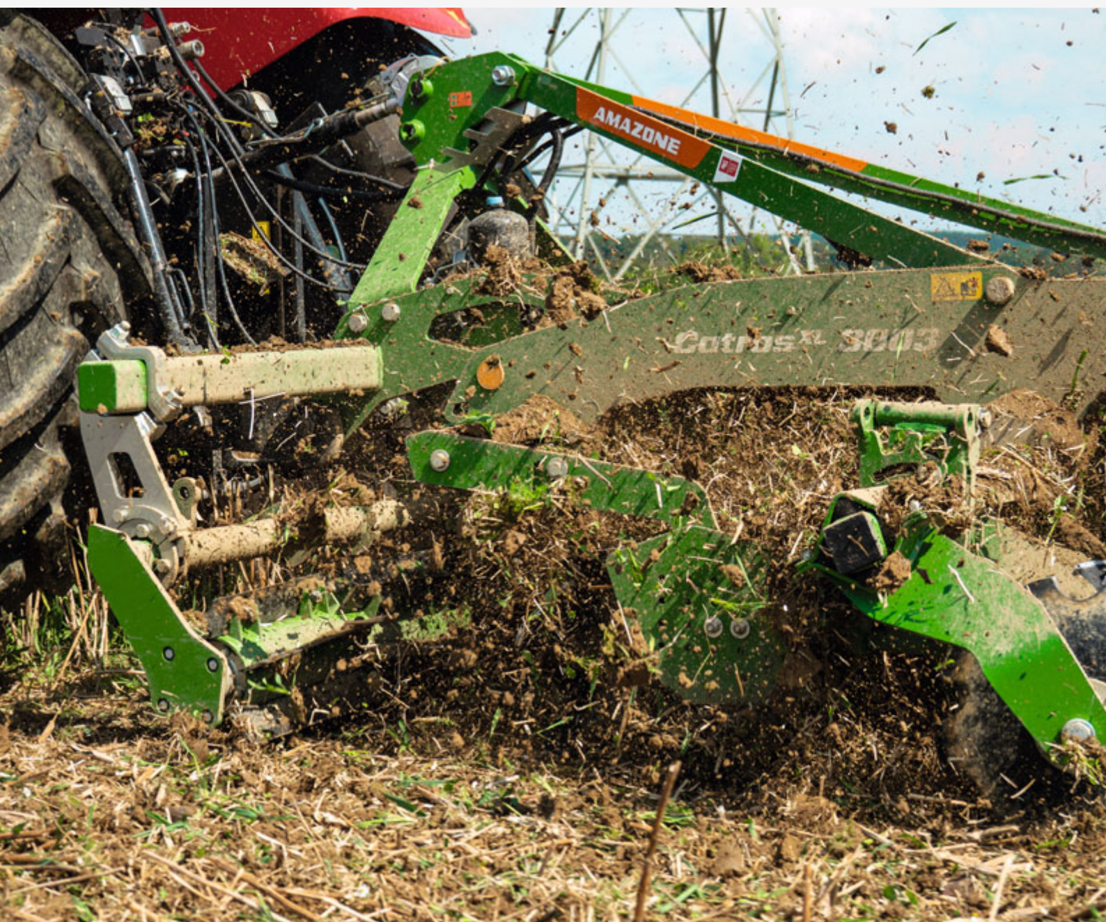
Ultra-shallow and intensive mixing of the soil and cutting the crop residue in combination with the knife roller
