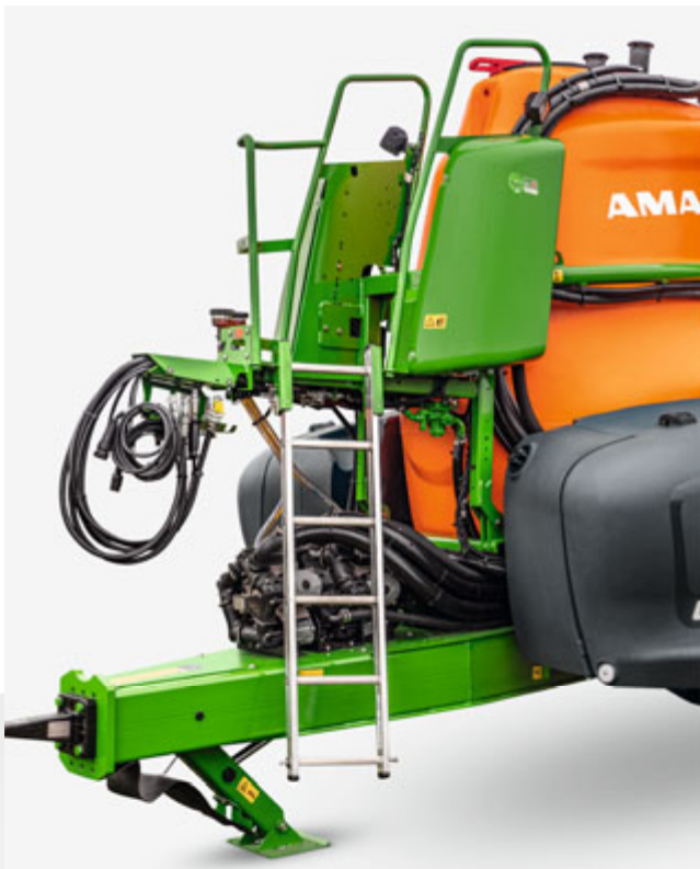
Safe access to the tank opening via the large platform
