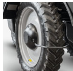
Drive wheel gearbox cover and crop divider on the Pantera 4504-HW
