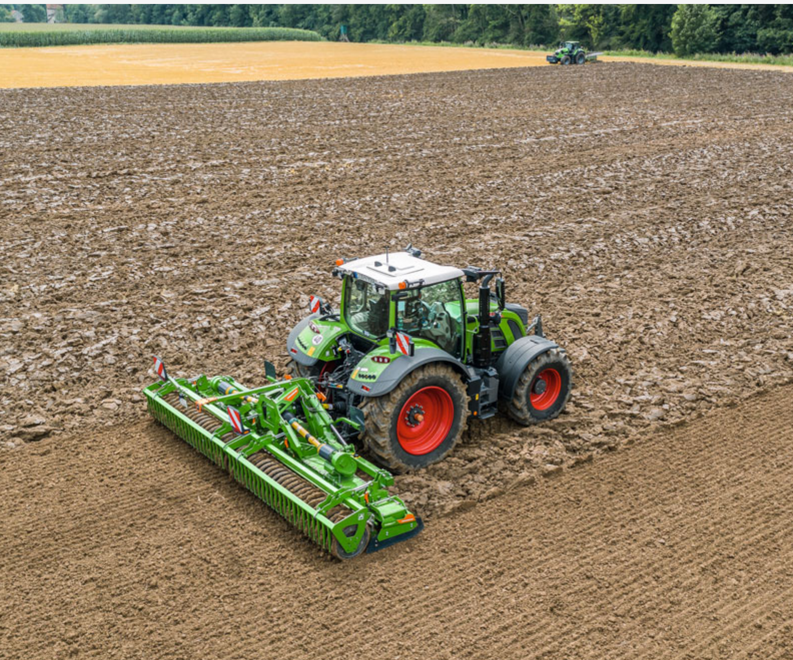
KE 6002-2-400 with Rotamix system for use after inversion soil tillage
