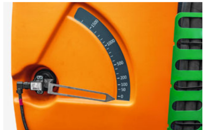
Fill level indicator clearly visible from the tractor
