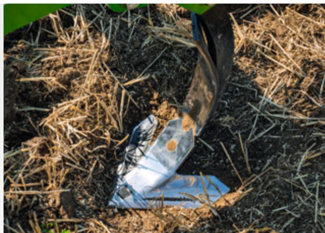
The extensive AMAZONE C-Mix share range now includes a 320-mm-wide duckfoot share for shallow, full-surface soil tillage.
