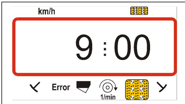
The first figure shows the dialed mode "9", the second figure "00" means that the seed drill is not equipped with an additional drive.
