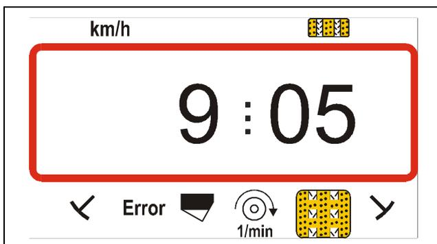
The first figure shows the dialed Mode "9", the second figure "05" means that after having pressed key the additional drive switches on for a period of 5 seconds and thus already provides a seed pre-metering before the seed drill starts to travel. The period to be seed depends on the driving behaviour of the tractor operator in the headlands and can be set between 0 and 98 seconds (please also refer to
