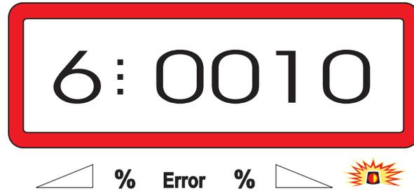
The first digit shows the chosen mode "6", the second the average forward speed in [k.p.h.] – e.g. "0010" for 10 k.p.h..
