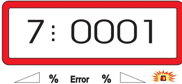
The first digit shows the dialled mode "7", the second indicates whether the broadcaster is equipped without "0000" or with weigh cell "0001" – here "0001" for broadcaster with weigh cell.
