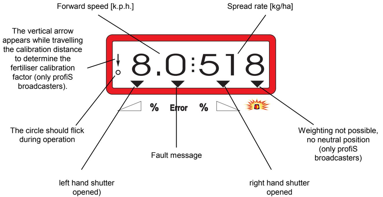
Operating display after pressing the keys for the common spread rate change (+10%)
