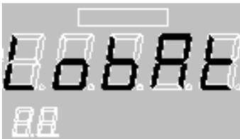
Low supply voltage. Check the battery of the tractor, the connections and the electric system.
