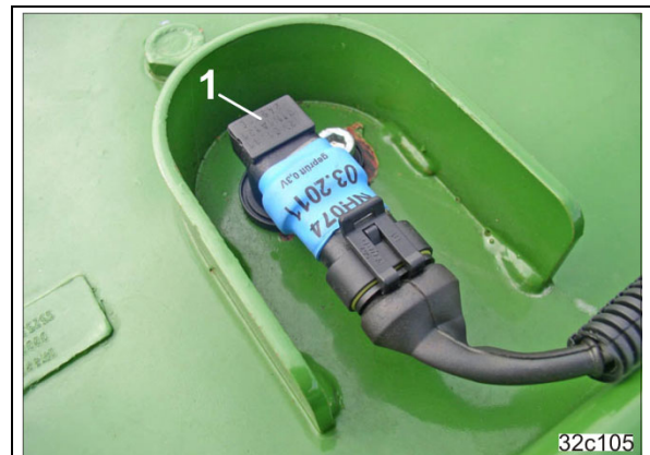
Hall sensor (1) on an angular gearbox
