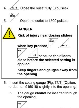
Increase the current offset by 5 pulses until the gauge fits exactly in the opening (Fig. 77).
