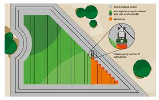
Position-dependent, automatic on/off switching for accurate placement of the seed
