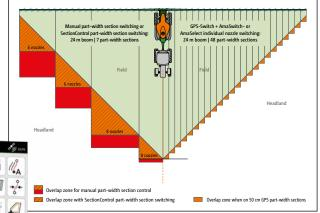
Up to 85% less overlap on the headland in comparison to conventional SectionControl partwidth section switching
