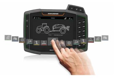
Automatic display of the buttons on the right-hand side of the screen via the proximity sensor
