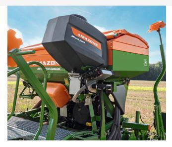
The Micro plus hopper can be easily accessed via the loading board
