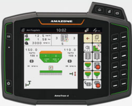
AMAZONE ISOBUS terminal AmaTron 4 with 8” touch screen
