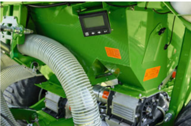
Primera DMC with electric metering drive and TwinTerminal 3.0
