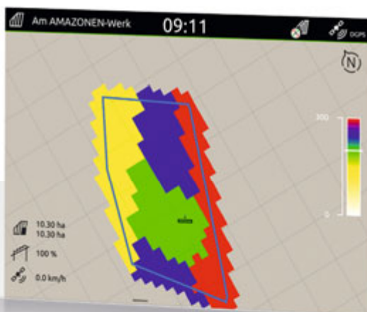
Display of the application map in AmaTron 4
