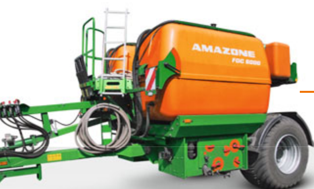
FDC 6000 Additional pulling power requirement of 50 hp
