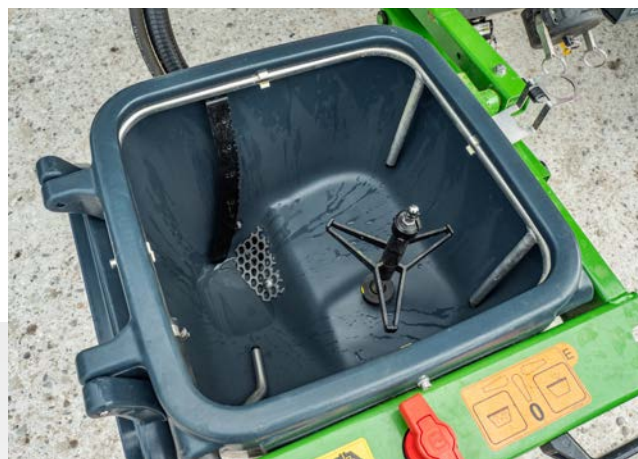
The high-performance induction bowl ensures minimum filling times and a homogeneous spray agent mixture
