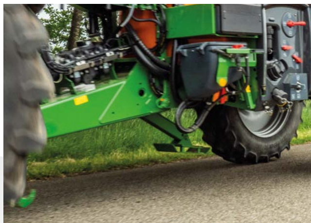
Lower mounted drawbar with hydraulic parking jack
