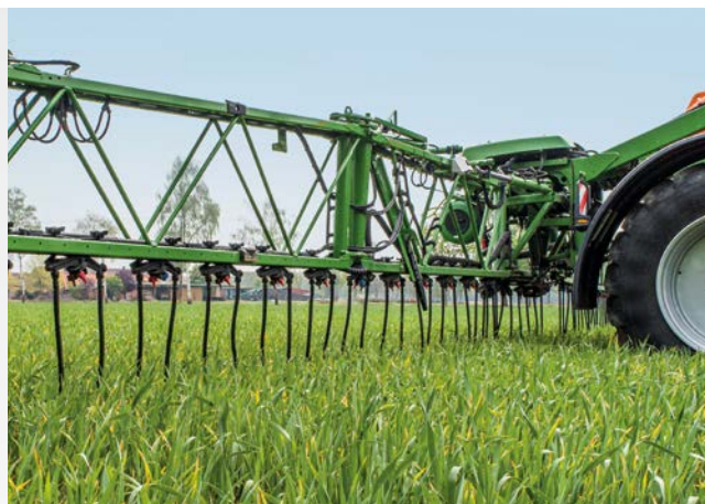
Drag hose equipment with an AmaSwitch 4-fold nozzle body and an extension kit on the Super-L2 boom.
