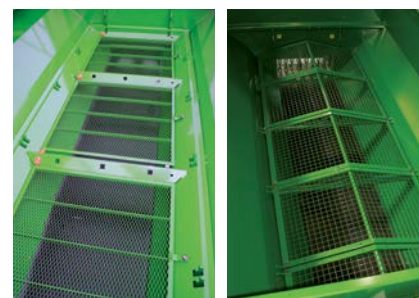
Large protective sieves – the spreading system is optimally protected from stones or other foreign objects.
