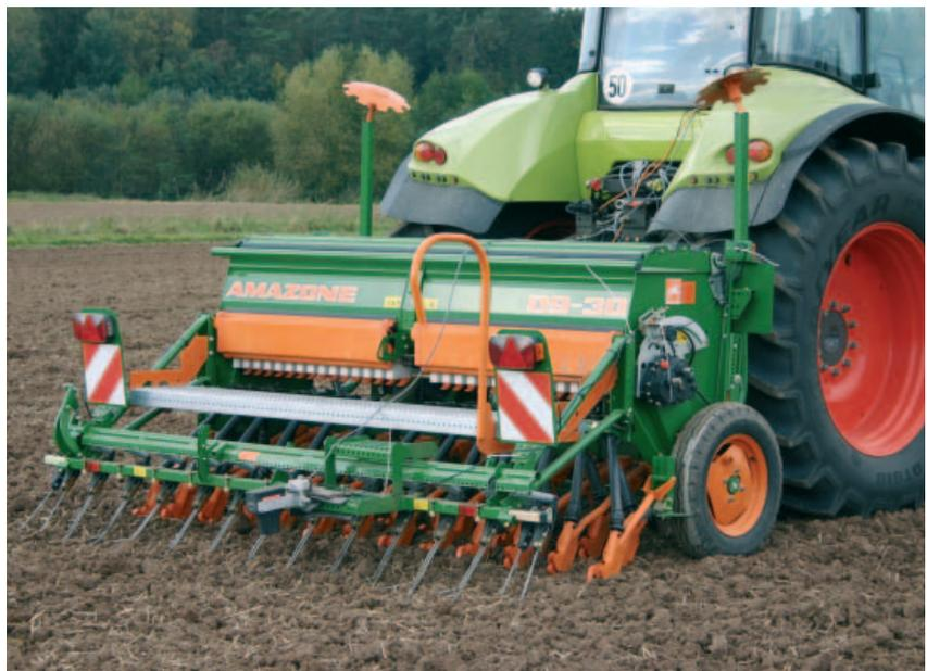
The 3 metre mounted seed drill had to show whether the set seed rates could be, in fact, maintained and how uniform the lateral distribution was.
