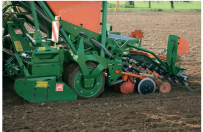
The press rollers enhanced the field germination by 5 to 10% under normal to dry conditions as the coulters also ran more smoothly with the placement depth being more uniform too.
