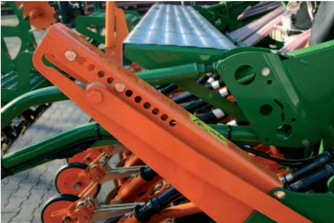
Advantage: The central setting of the coulter pressure is carried out comfortably on the right-hand side of the machine as viewed in the direction of travel. Disadvantage: The adjustment of the press rollers and depth-limiter discs is somewhat awkward, in contrast.
