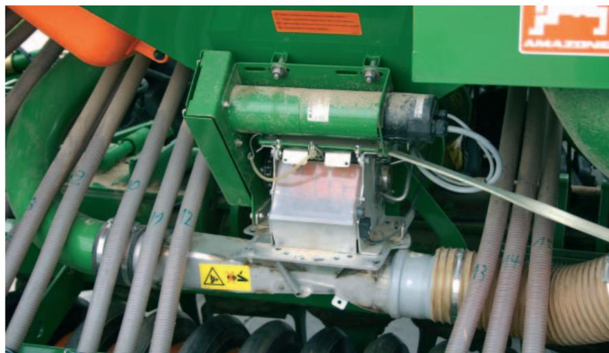
Advantage: The calibration operation requires little time. Disadvantage: the metering cassette and the facility for removing the remainder in the hopper are awkward to reach.
