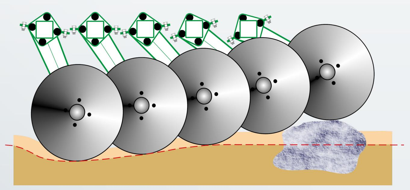
The **elastic sprung rubber buffer** blocks for suspending the discs, not only ensure optimum contour following, but also act as overload safety protection on each individual disc. The oversized rubber buffers are maintenance-free.
