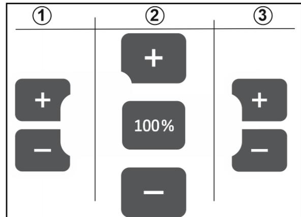
Work display while driving when the spread rate is changed on one side or both sides:
