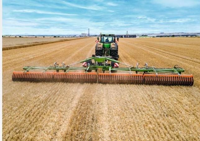
Instead of the harrow, the tool carrier can, as an alternative, also be equipped with various different rollers for good reconsolidation
