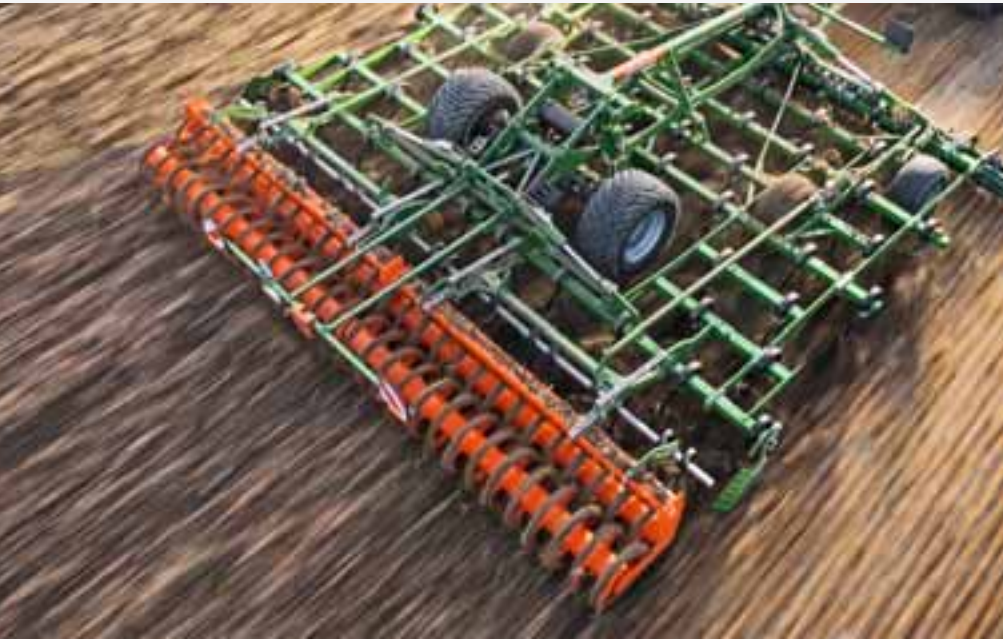
Cobra 7002-2TX in use for stubble cultivation
