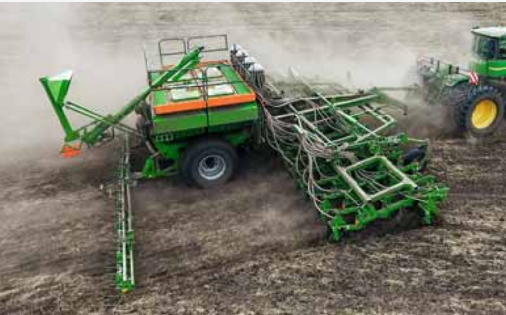
Primera DMC 12001-2C, 12 m working width with external distributor heads
