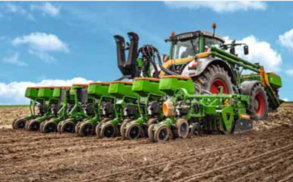
Precea 6000-2AFCC precision air seeder with 6002-2 Super rotary cultivator
