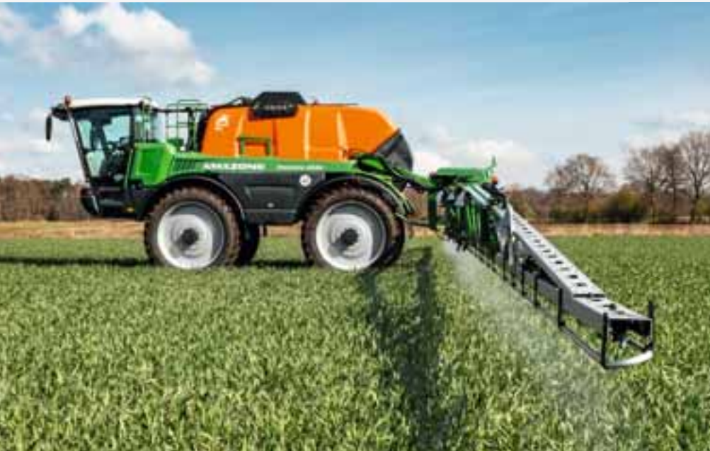
Pantera 4504 self-propelled sprayer with a ground clearance of 1.2 m
