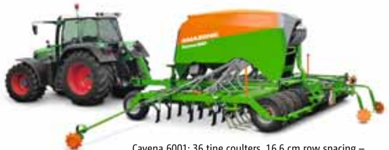
Cayena 6001: 36 tine coulters, 16.6 cm row spacing – forward speeds of up to 15 km/h
