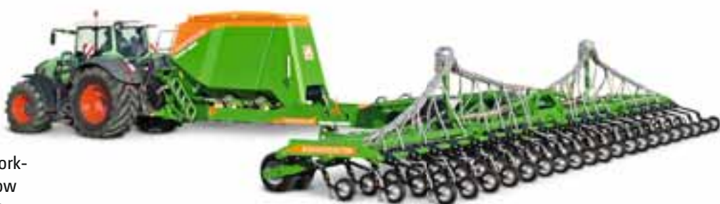
Condor 15001-C: wide in the field, narrow on the road with 3 m transport width
