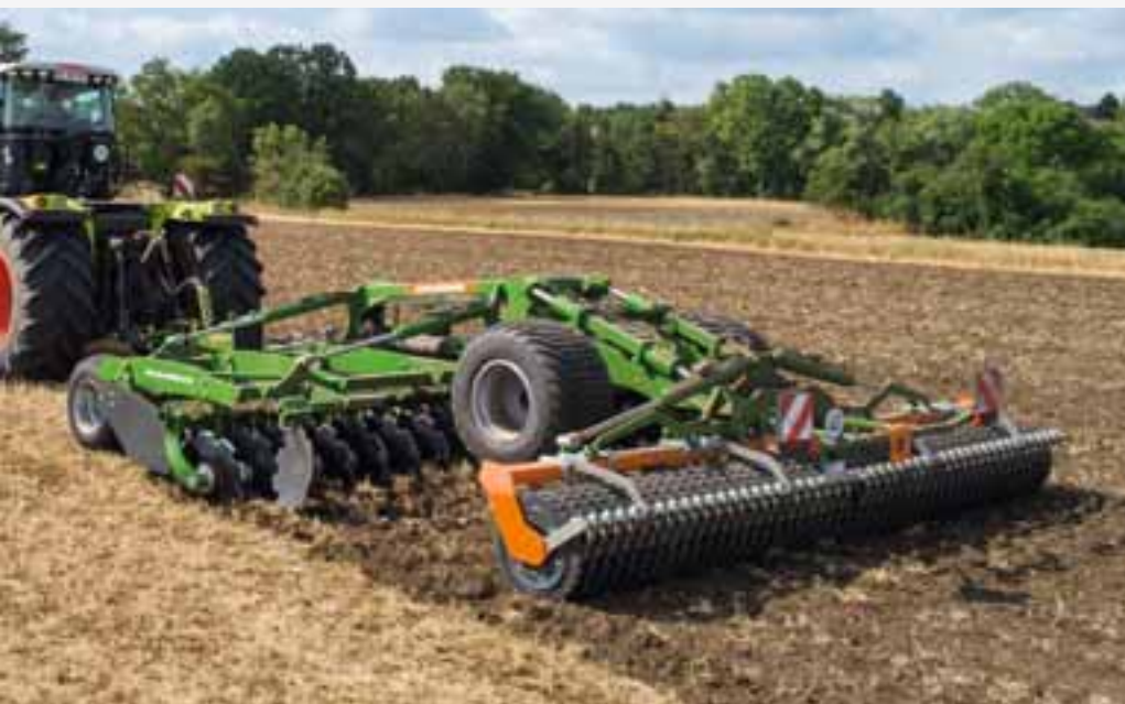
Certos 6002-2TX in 6 m working width with TX central running gear
