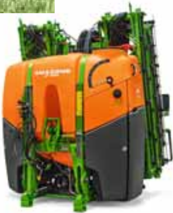
UF 1602 mounted sprayer with 28 m Super-S2 boom
