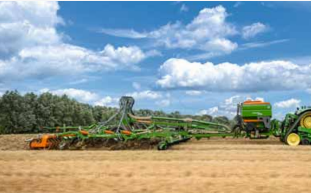
XTender 4200 with Cenius 7003-2TX and two conveying systems to deliver fertiliser and seed
