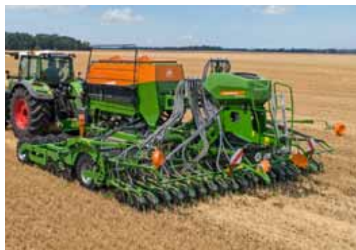
Cirrus 6003-ZCC with Minimum TillDiscs – minimal, water-conserving soil tillage
