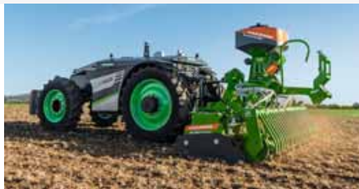
4-wheel AgXeed AgBot and AMAZONE KE 3001 Super rotary harrow with Green-Drill harrow-mounted catch crop seeder box
