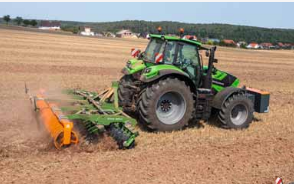
Catros + 5003-2 with serrated discs and a working width of 5 m
