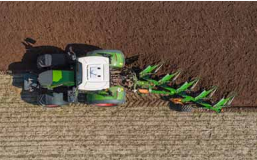
Teres 300, 5 furrow stepped adjustment plough
