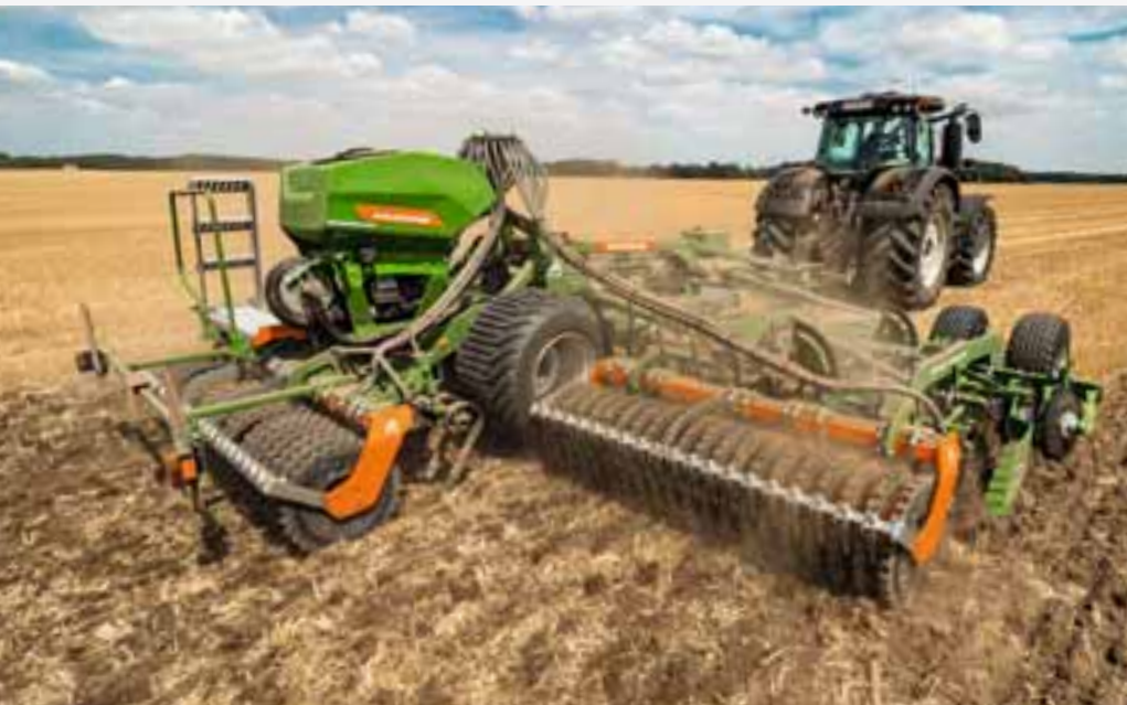
Catros XL 8003-2TX compact disc harrow with GreenDrill 501 universal catch crop seeder box
