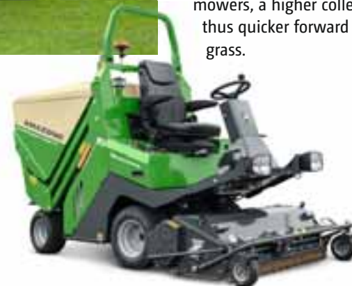
Profihopper 4WDi SmartLine with front wheel drive and a 0-radius turn
