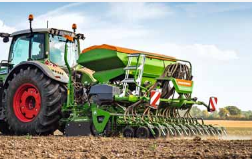
Centaya 3000 Super with TwinTeC double disc coulters
