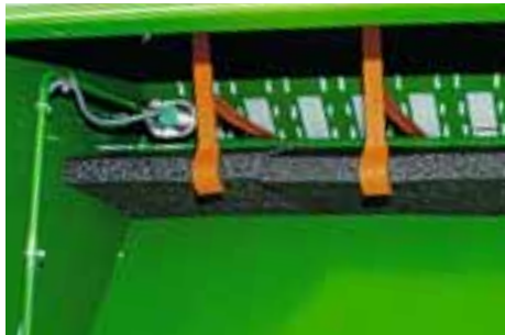
An optional rape insert kit can be quickly and easily attached inside the seed hopper to reduce the residual seed volumes.
