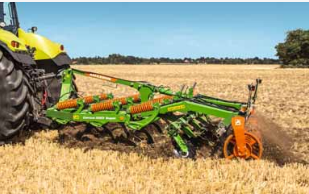
Cenius 3003 Super with U-Profile roller
