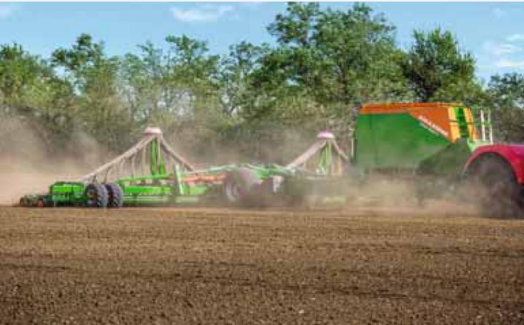
Citan 12001-C, with a split, three-chamber hopper as standard
