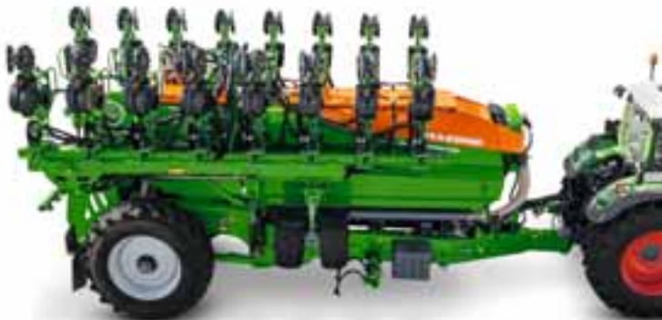
Precea 12000-TCC folded to 3 m transport width
