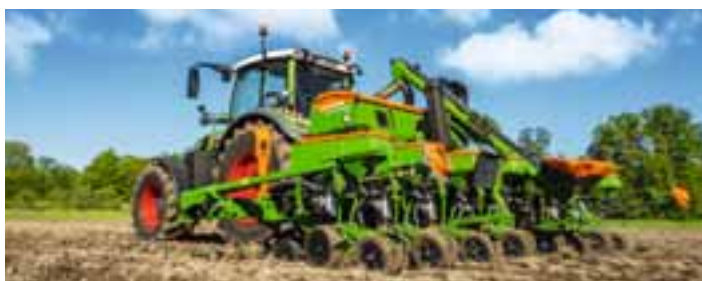
Precision seeding: e.g. Precea 6000-2CC precision air seeder
