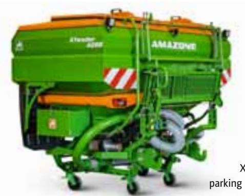
XTender 4200 with Cenius 7003-2TX and two conveying systems to deliver fertiliser and seed
