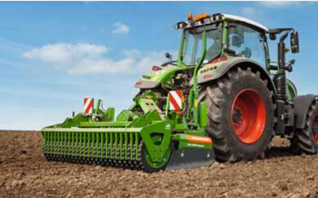
KG 3001 rotary cultivator with wedge ring roller with Matrix tyre profile
