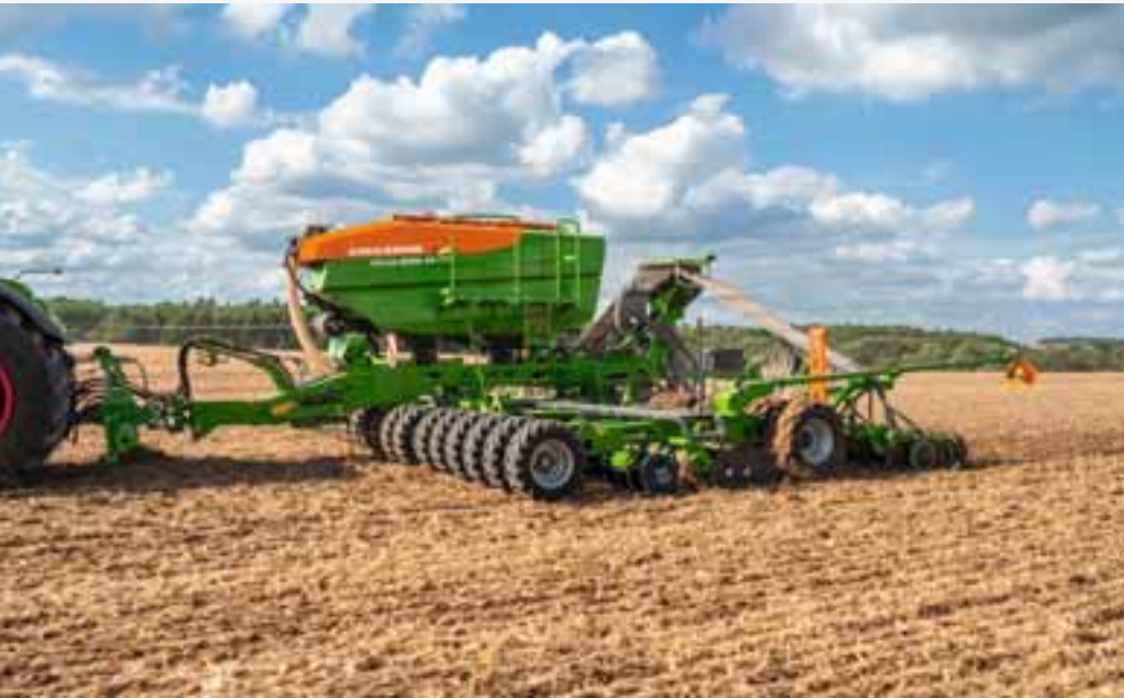
Cirrus 9004-2C Grand with wheel mark eradicators in catch crop establishment
