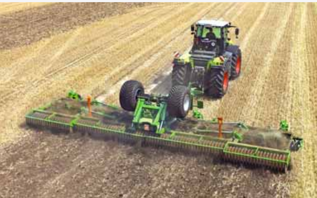
The 12 m wide Catros + 12003-2TS seen here stubble tilling
