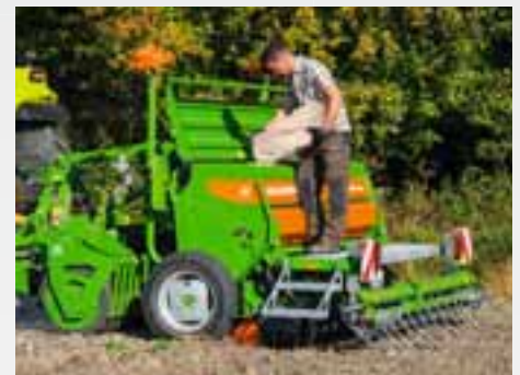
D9 3000 Super with a 3 m working width and the standard WS coulters
