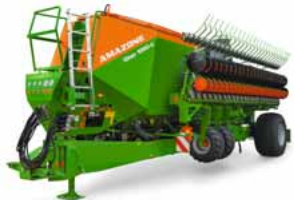
Citan 12000-C folded to 3 m transport width
