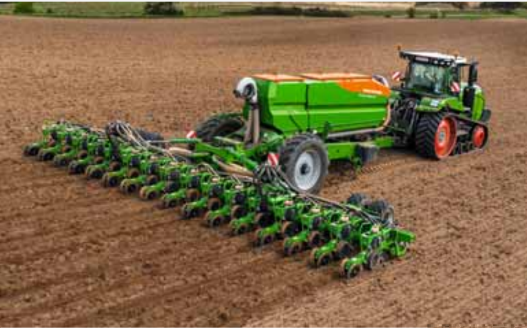
Precea 12000-TCC in a working width of 12 m and 16 rows
