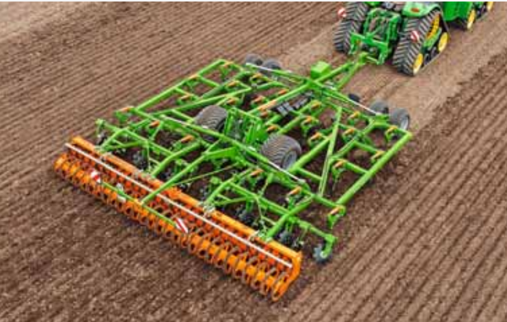
Cenius 4003-2TX Super with wedge ring roller
