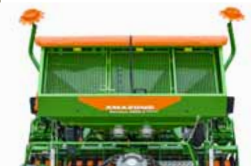
Centaya 4000-C Special with a split, twin-chamber tank in the ratio of 70:30. This enables two different materials to be metered separately.
