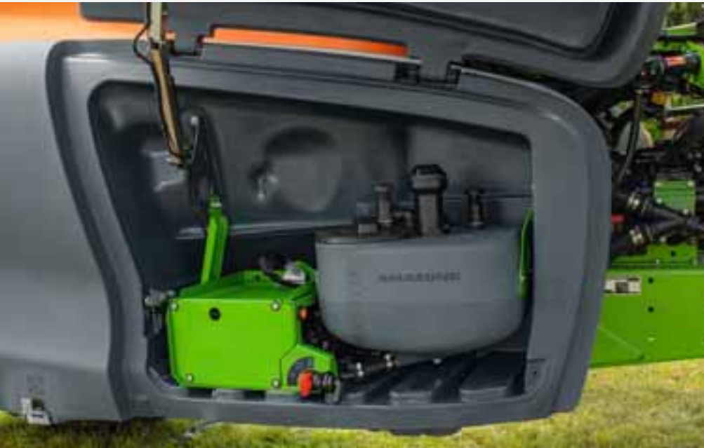
DirectInject equipment with 50 l tank and pump unit in the storage compartment of the UX 01 Super
