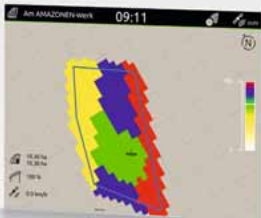
Display of the application map in AmaTron 4
