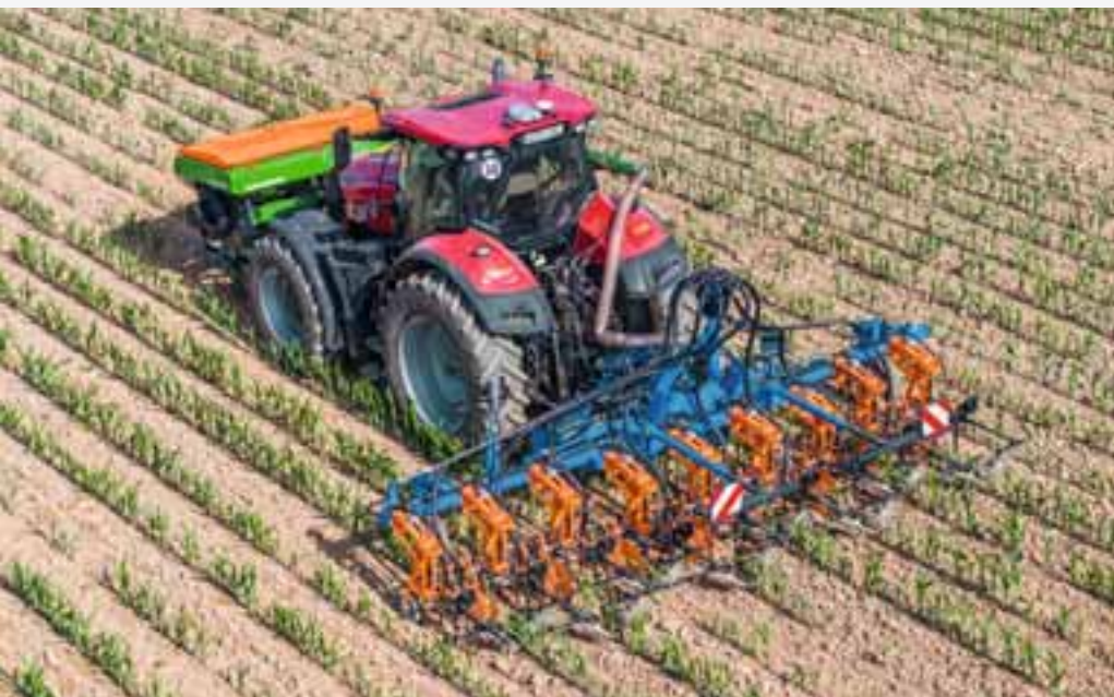
Venterra 2K in combination with the FTender front mounted hopper for row fertilisation
