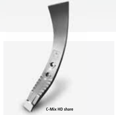
One-piece C-Mix HD share 80 mm: hard-wearing variant (HD – Heavy Duty) with hard metal plates in the main wear zones.
