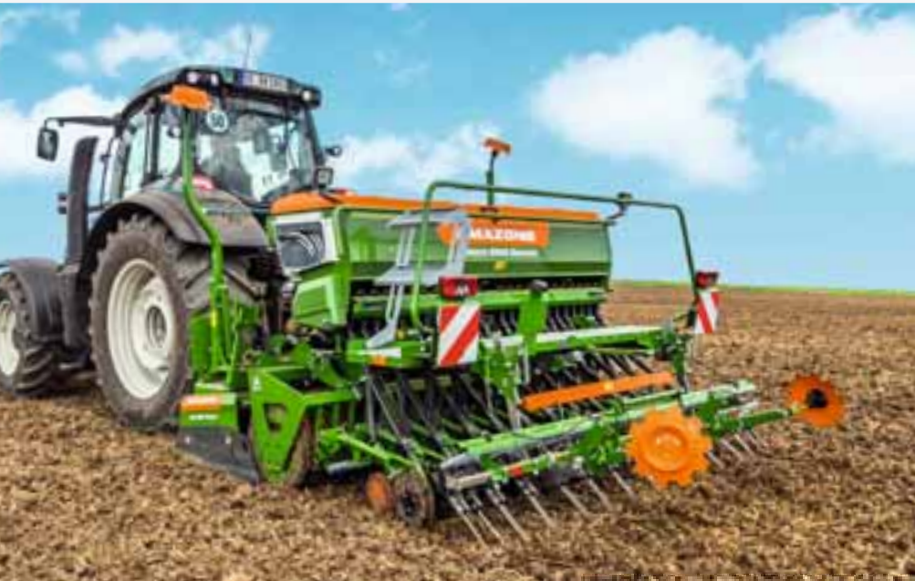
Cataya 3000 Special with RoTeC coulters and Exact following harrow
