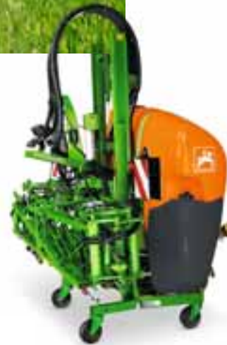
UF 1201 with 15 m Super-S2 boom
