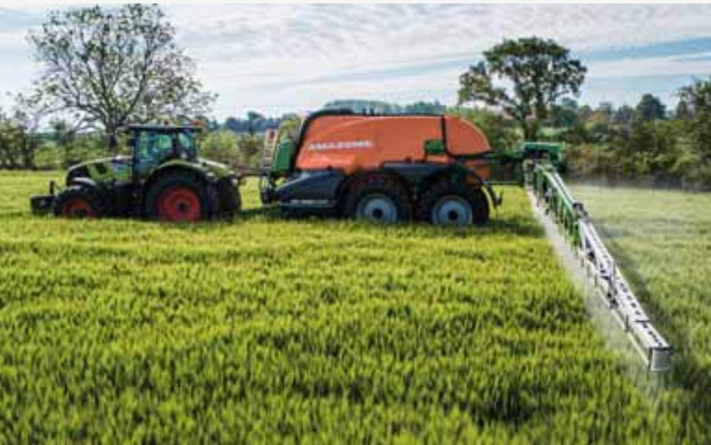
UX 11201 trailed sprayer with 40 m Super-L2 boom
