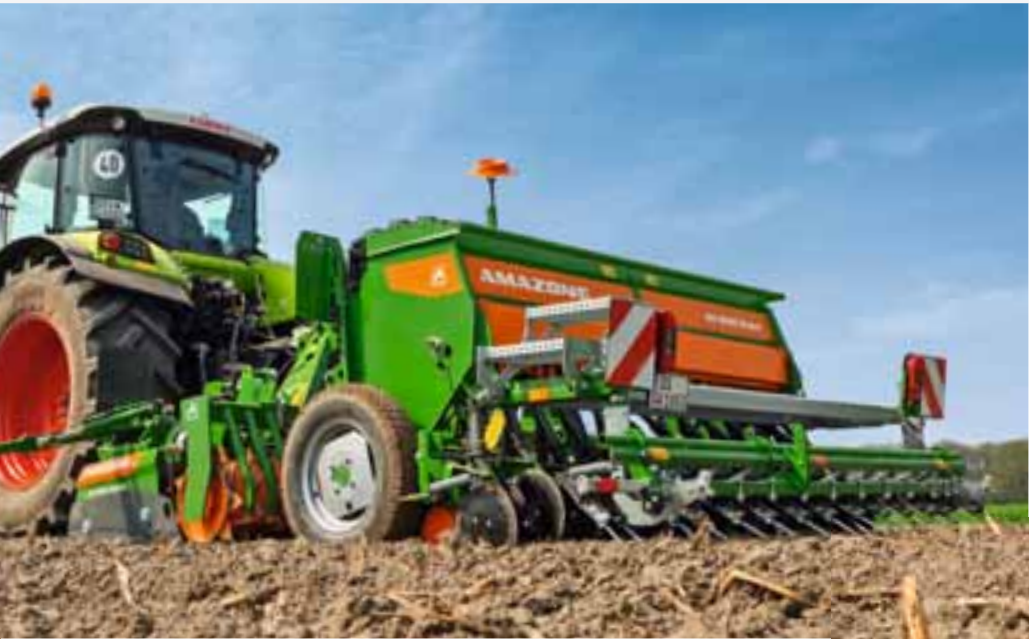
D9 3000 Super with Exact following harrow in combination with rotary harrow and tooth packer roller
