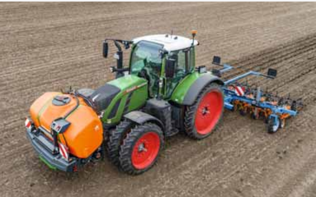
FT-P 1502 front tank in action with a SCHMOTZER hoeing machine for band spraying
