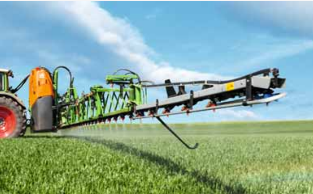
UF 2002 mounted sprayer with 30 m Super-S2 boom
