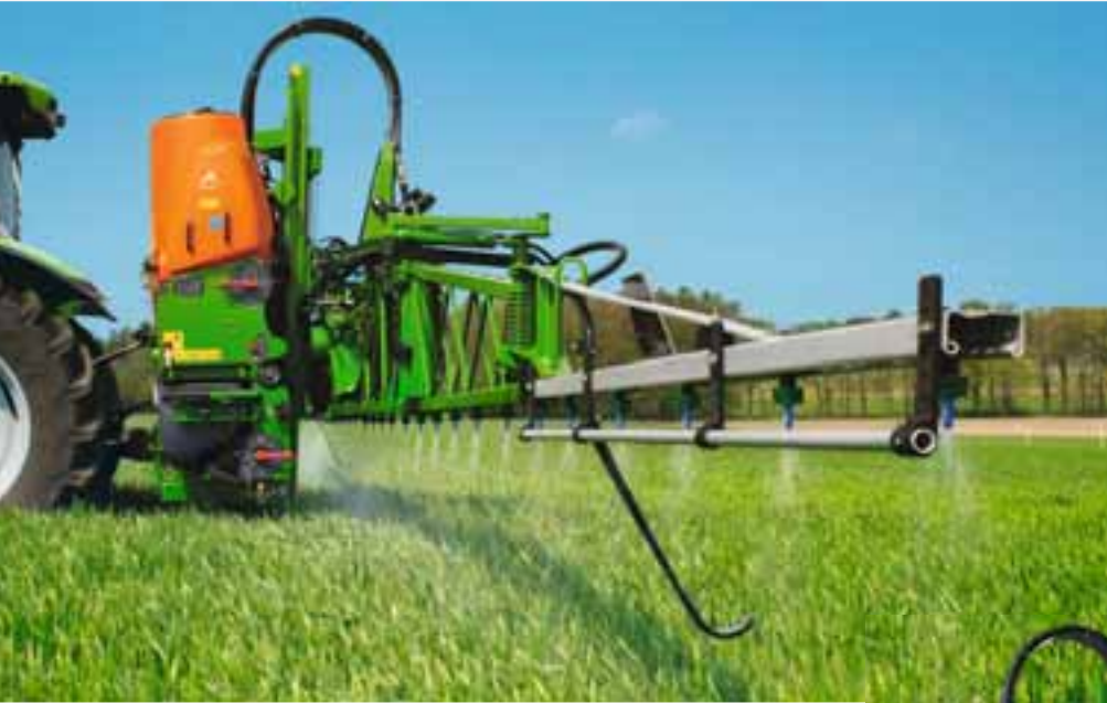
UF 1201 mounted sprayer with 18 m Super-S2 boom
