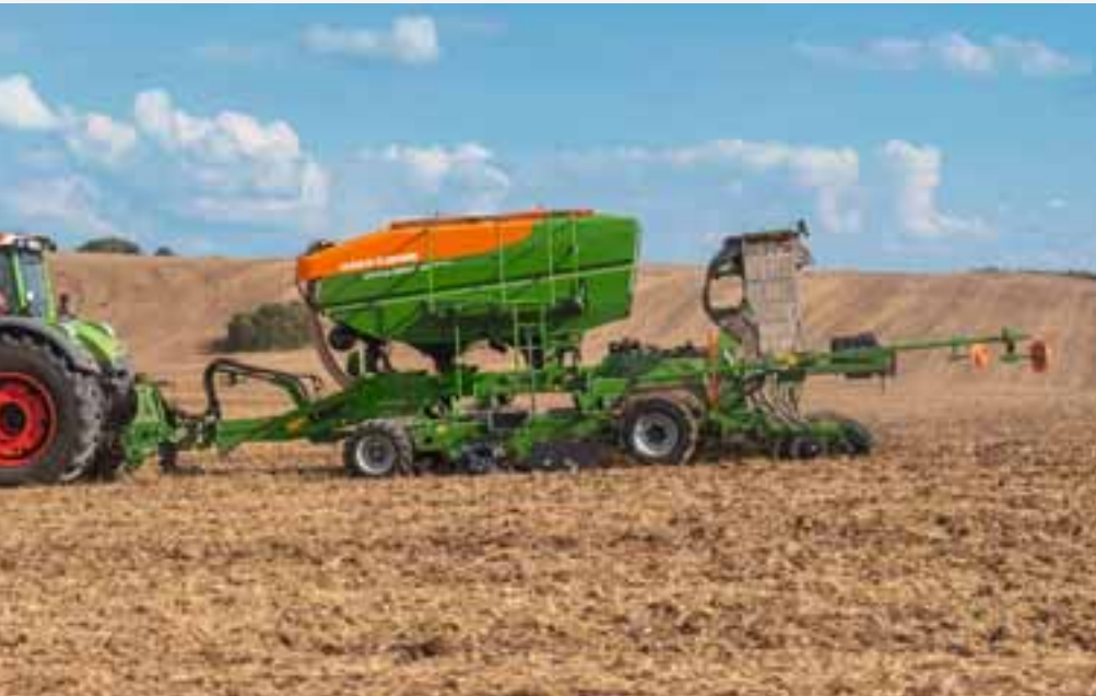
Cirrus 9004-2C Grand with matrix tyres for strip-wise reconsolidation.
