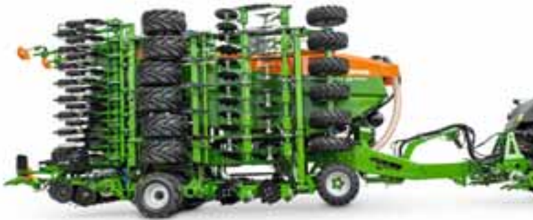
Cirrus 9004-2C Grand folded to a transport width of 3 m
