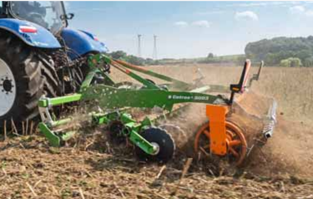
Catros + 3003 with serrated discs in a 3 m working width
