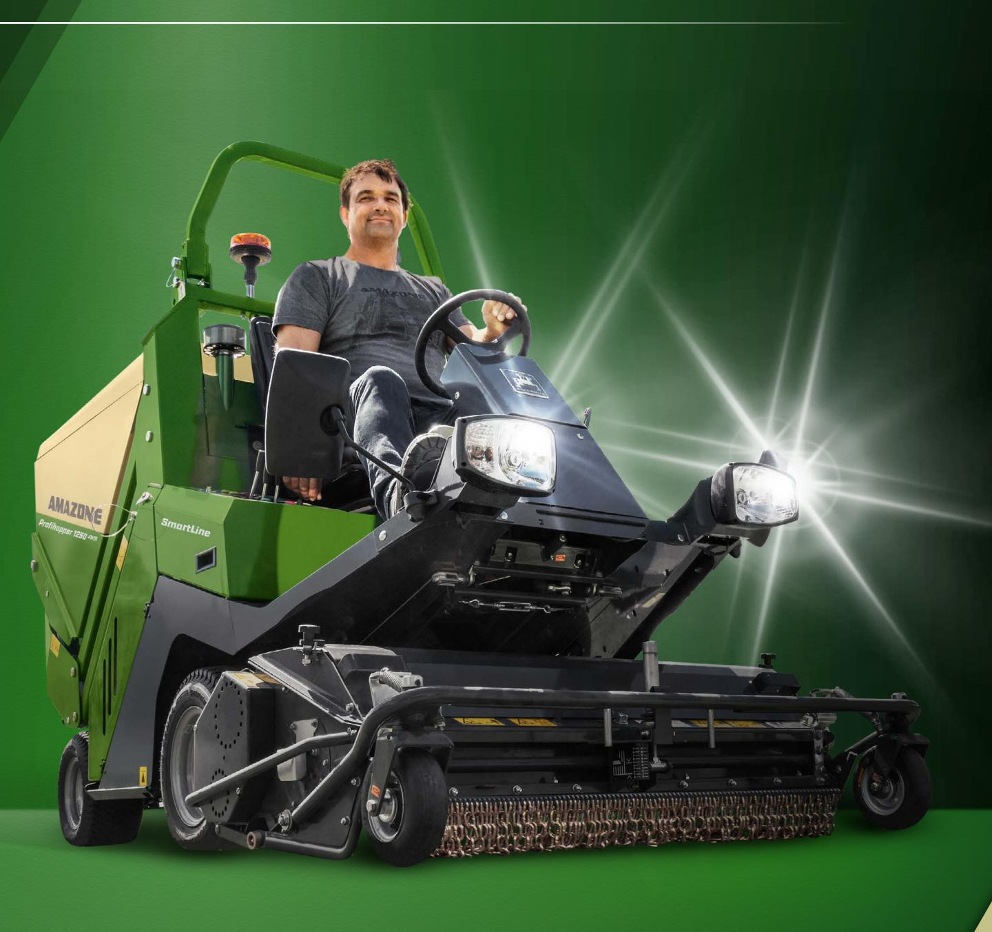
The Profihopper is not bothered whether the grass is dry or wet, exceptionally tall or even thick, it always achieves first class results. This is because the SmartCut exact cut rotor ensures outstanding cutting and collecting quality and the PowerCompactor collecting and conveying system, consisting of a longitudinal and a cross conveying auger, ensures the maximum area coverage under any conditions.
