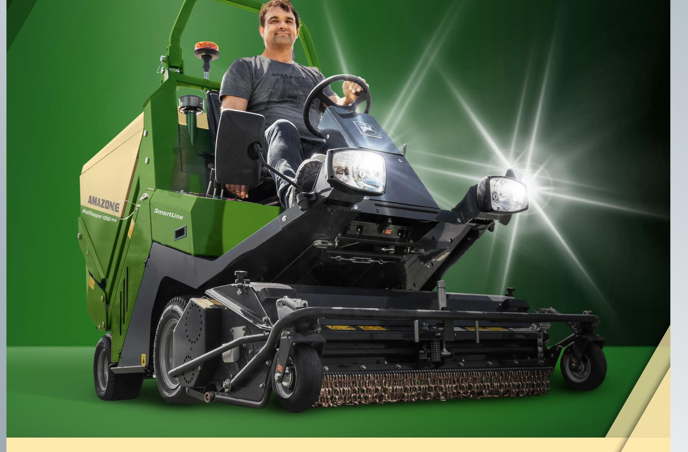
The Profihopper is not bothered whether the grass is dry or wet, exceptionally tall or even thick, it always achieves first class results. This is because the SmartCut exact cut rotor ensures outstanding cutting and collecting quality and the PowerCompactor collecting and conveying system, consisting of a longitudinal and a cross conveying auger, ensures the maximum area coverage under any conditions.
