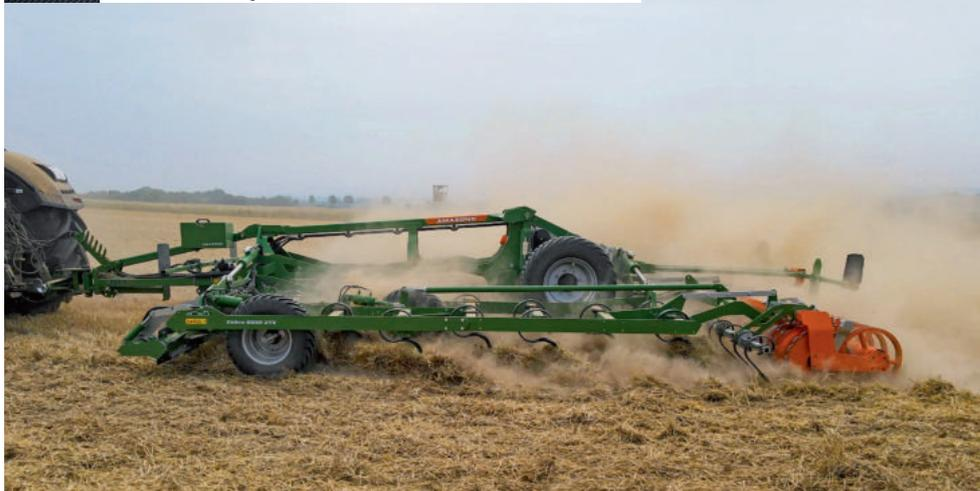
The 45 leaf-spring tines are actually arranged on 8 bars. The bars are spaced at 50-70cm, underbeam clearance is 60cm.
