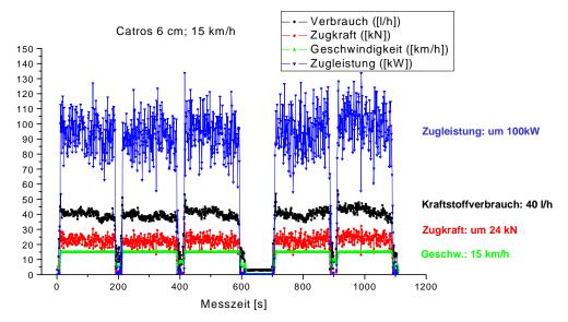
Picture 2: Graphic illustration of a measuring travel
