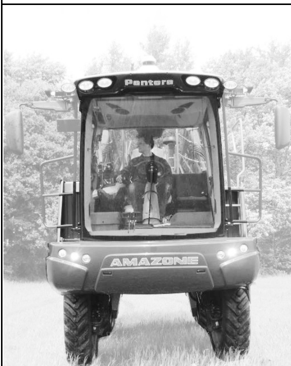
Machine lowered (default position)
