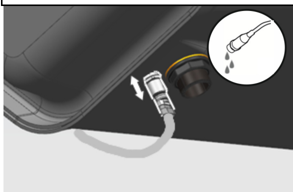
Flushing water tank pressure sensor underneath the flushing water tank
