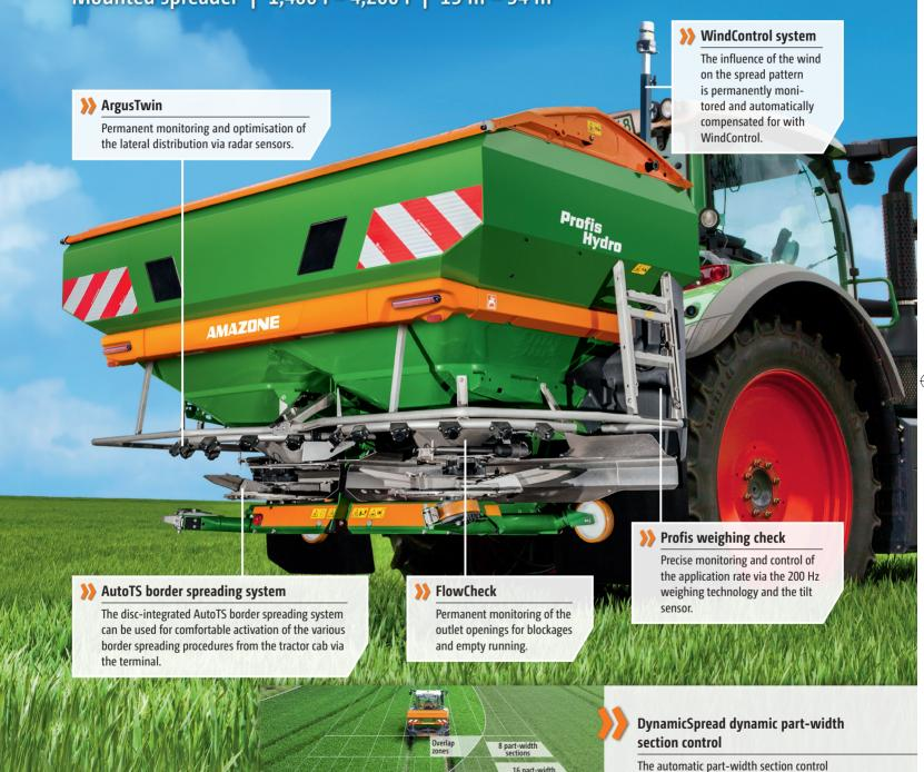
with up to 128 part-width sections in the form of a kidney-shaped pattern guarantees high precision switching in wedge shaped fields or at the headland. Outer part-width sections can also be controlled.
