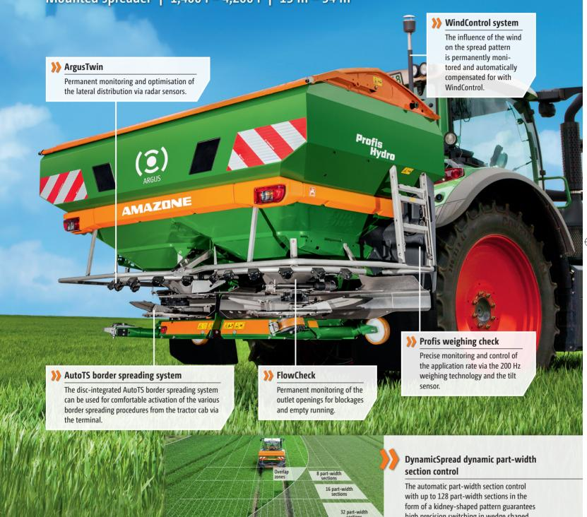
high precision switching in wedge shaped fields or at the headland. Outer part-width sections can also be controlled.
