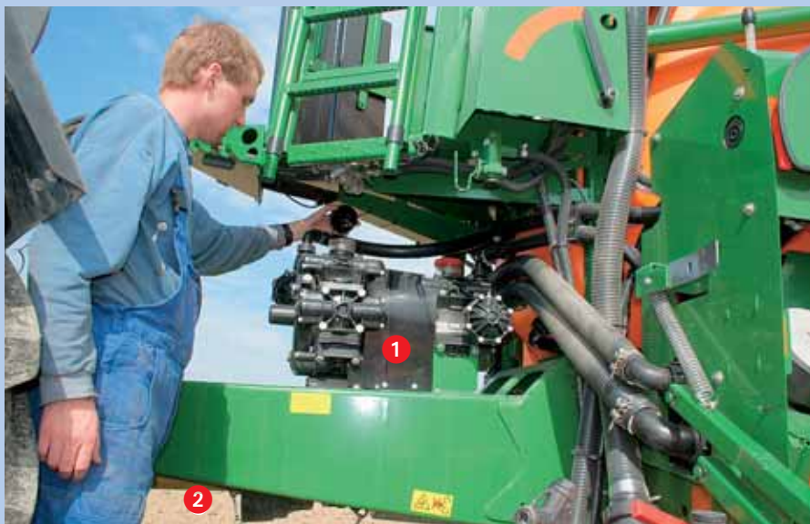
The pump double-pack (1) at 250 + 180 l/min is standard. Driving it from underneath (2) increases the ground clearance.
