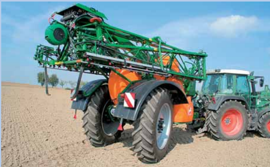
The optional axle steering for 5750 € increases mobility without losing stability – superb.
