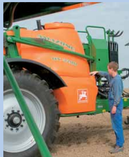
The 320 l clear water tank is easy to fill – with a hose connection even on the left. However, it obscures the driver's view of the tyres.
