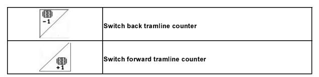
The tramline counter switches when the machine is raised.
