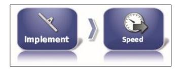
When the ISO ground speed is enabled, the speed is transmitted to the implement through the ISOBUS protocol.
