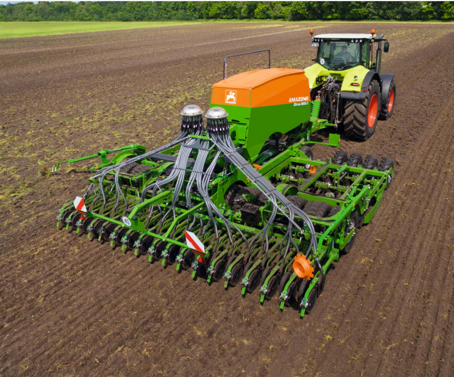
Cirrus 6003-2 trailed sowing combination with TwinTeC + double disc coulters
