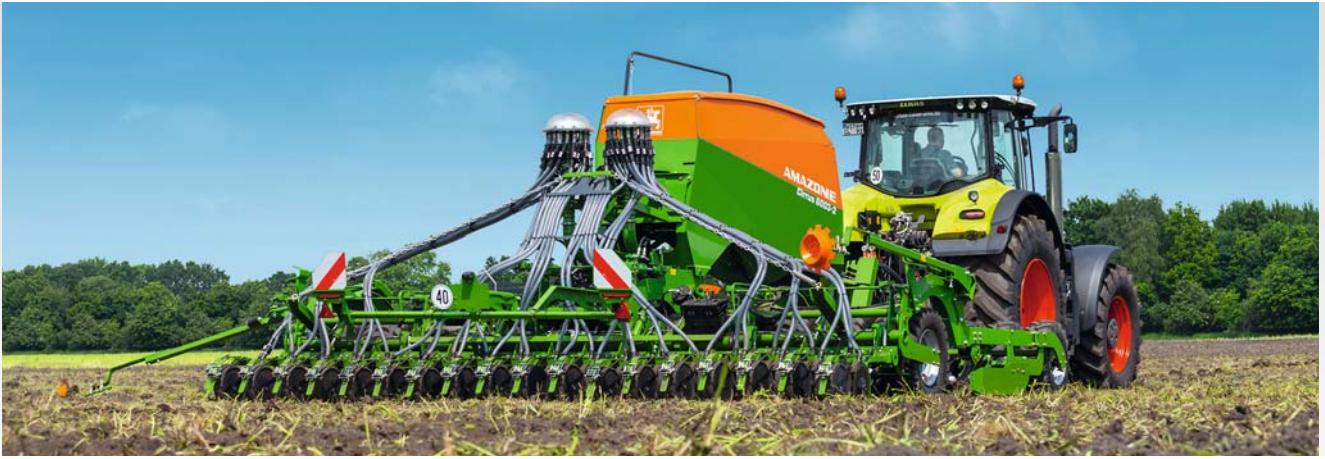
Cirrus 6003-2 trailed sowing combination with TwinTeC + double disc coulters
