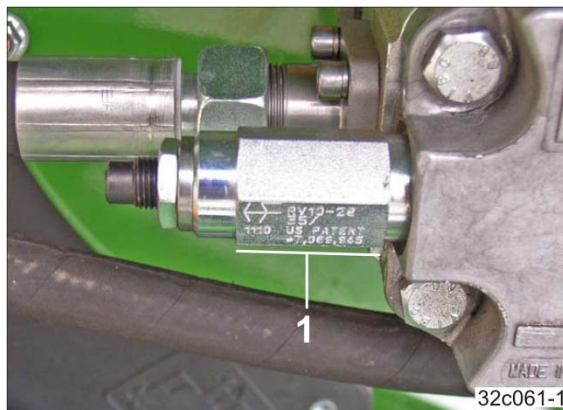
Pressure relief valve with hexagonal outer contour (1)
