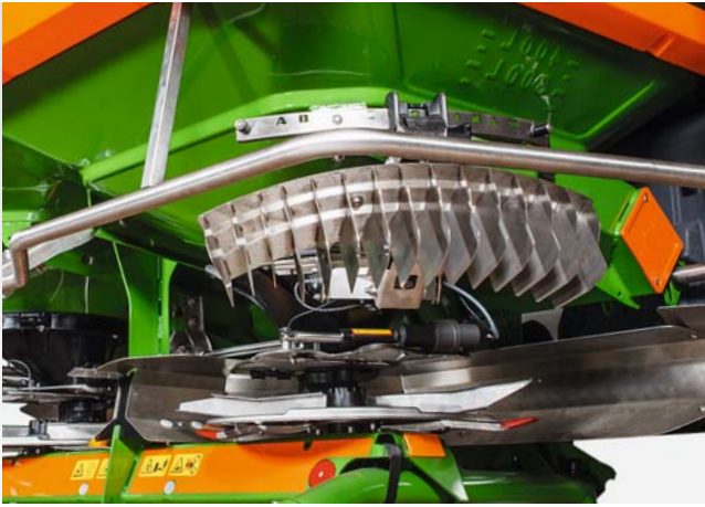
Limiter V + electric border spreading system
