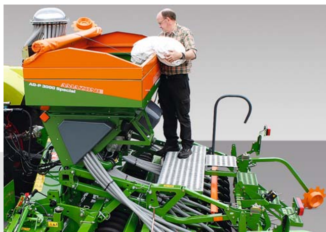
An especially-wide loading board eases filling
