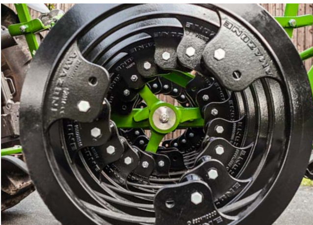
Sufficient space is created by the lack of the centre axle
