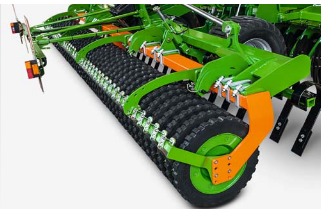
KWM 650 wedge ring roller with matrix profile
