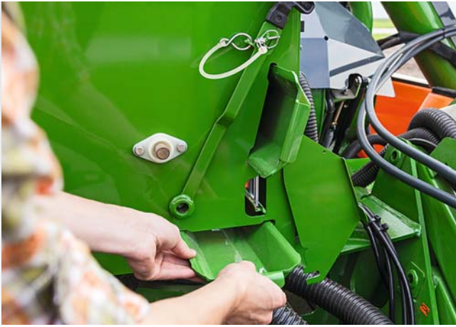
Calibration trays which can be pulled out on the left hand side
