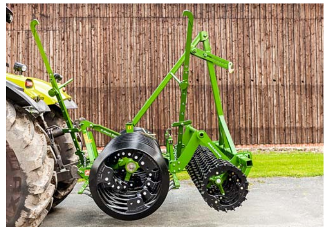
C-Pack 900 with NW breaker ring roller in the transport position
