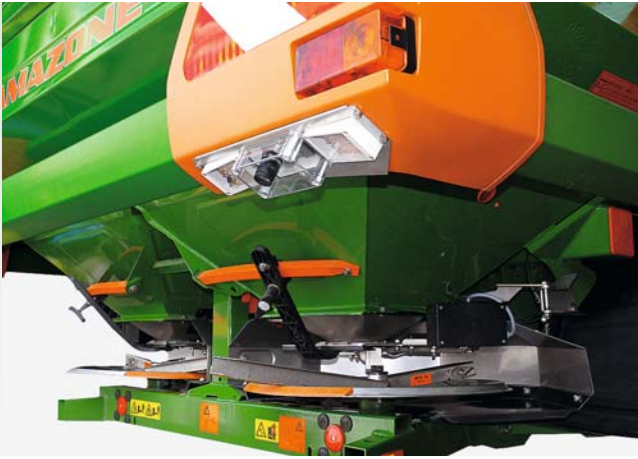
Argus System 2007 for automated mineral fertiliser application
