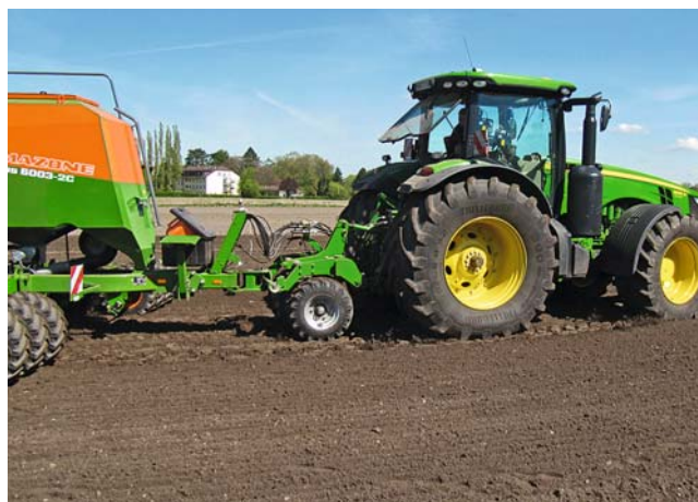
T-Pack U intermediate axle packer (universal)
