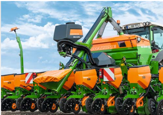
Filling auger for filling the rear fertiliser tank
