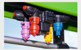
If AmaSelect and GPS-Switch are combined, part-width sections at a spacing of 50 cm can be controlled individually and this keeps the overlap zones down to a minimum. This is optimum, both from an economic and also an ecological point of view.
