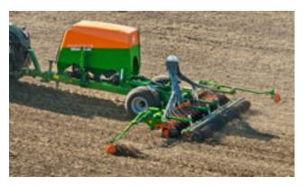
In a split operation, the second cultivation and the sowing pass are carried out separately – and, depending on the local conditions, with more or less a timely operation.
