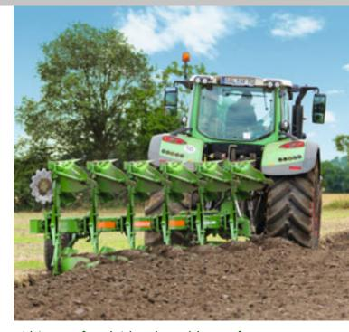
With its 83 cm frame height and smooth beam surface, the Cayron ensures especially good trash passage.
