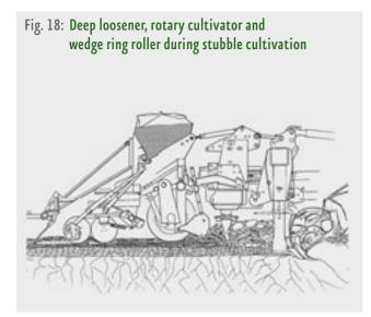
implement always at the same point. In case of dry soil conditions the combination of rotary cultivator + wedge ring roller + precision single seeder can be used after conventional and conservation primary tillage.
