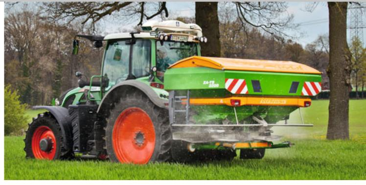
Fertiliser spreader and N-sensor for site-specific fertilisation.
