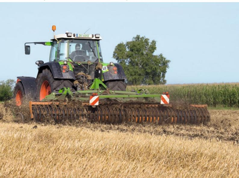
vating discs level the soil and at the same time provide some loose soil which is then firmed again by the wedge ring tyres.
