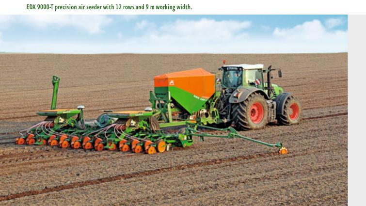
conventional precision air seeders. The EDX complete programme includes 3 three-point mounted machines in a 6 m working width and two trailed machines in 6 m and 9 m working widths. With its comprehensive range, the perfect machine for all relevant farming applications is available.
