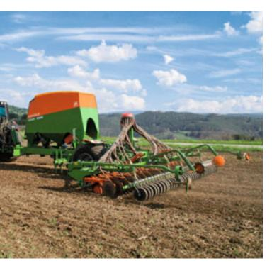
The Citan 6000, in a working width of 6 m, for operation with tractors from 120 HP.
