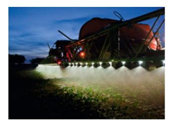
The work lights on the booms or LED individual nozzle illumination eases work after dark.
