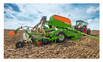
Cirrus is equipped with pre-cultivating disc elements and achieves daily outputs of 25 ha to 60 ha (depending on working widths of 3 m, 4 m or 6 m).
