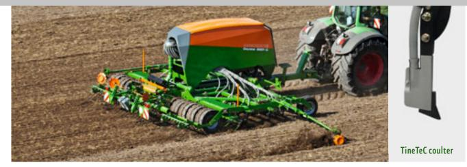
The Cayena, equipped with its TineTeC coulters, is suitable above all for sowing on hard and stony soils.
