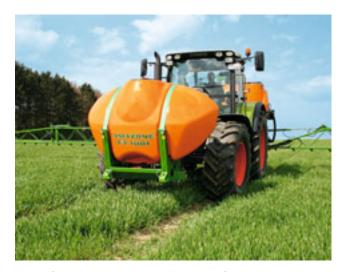
The FT front tank increases the capacity of the UF mounted sprayers by 1,000 l to 2,800 l max.
