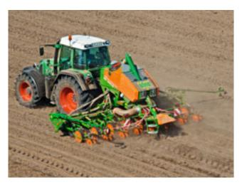
EDX 6000-2C with integrated fertiliser hopper, 8 rows and 6 m working width.
