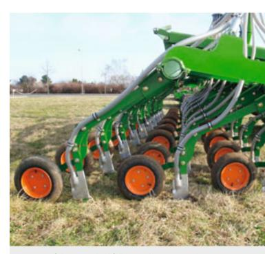
By means of the press wheel following the ConTeC coulters on the Condor, reconsolidation is achieved that ensures better seed-soil contact.
