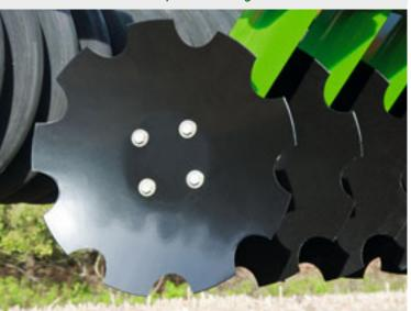
The range of application for the knife ring roller is in medium to heavy, clay soils and on sites where only few stones prevail.
