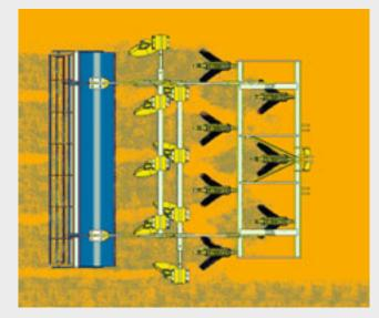
Fig. 5a: Poor straw incorporation and the simultaneous formation of swaths with a two row wing tine cultivator
