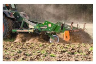
The task of the Cenius cultivator is to work the soils deeper.
