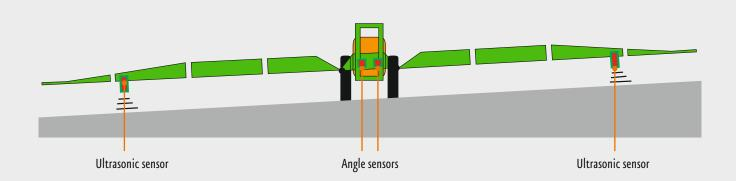
increasingly used to increase work rates. The multiplecushioned AMAZONE booms – supported by Distance-Control – allow these higher operating speeds, and as far as the equipment technology is concerned, to ranges even beyond 20 km/h.
