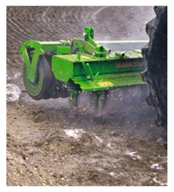
See the sparks fly – KG rotary cultivator in operation on the Hude stone torture track.
