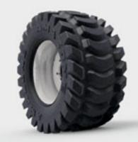
Thanks to the good wall flexing, the radial designed profile of the Matrix tyre virtually rests evenly on the soil across all the rows creating even germination conditions.
