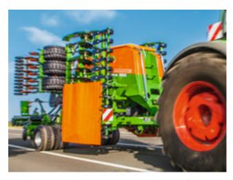
Both the Cirrus and also the Citan seed drills can be folded in to a transport width of 3 m in the shortest of time.
