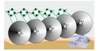
Fig. 3: Rubber sprung elements for stone safety on the Catros
