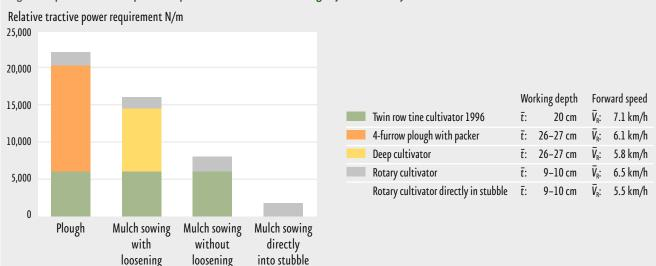
Fig. 37: Specific tractive power requirement for different tillage systems; loamy site
