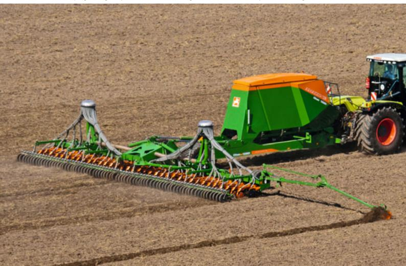
The Citan 12001-C and 15001-C offer the possibility to place, in addition to the seed, also fertiliser down in the seed furrow. For this reason, the hopper is divided and can be filled 2/3 with seed and 1/3 with fertiliser or a second kind of seed. If division of the tank is not necessary, it can be completely filled with one kind of seed. The metering is carried out via Vario gearboxes which can each meter seed rates of 2 to 400 kg per hectare.
