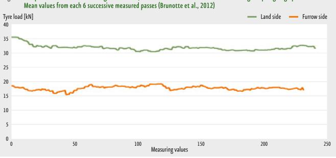
Fig. 24: Comparison of the wheel loading on land side/furrow side from rear tractor wheels during the ploughing operation. Mean values from each 6 successive measured passes (Brunotte et al., 2012)
