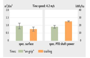
than in the reconsolidated area). Thus even large amounts of rainwater can drain away in the unrolled, loose areas. But be careful: on silty soils, the tine speed of any PTO driven harrow should be reduced by selectable speed gearboxes or engine revs because they are renowned for aggregates which are heavily prone to capping. After drilling the coarser aggregates from the unrolled areas are distributed over the entire field by means of a special harrow (Exact following harrow) (see Fig. 14).
