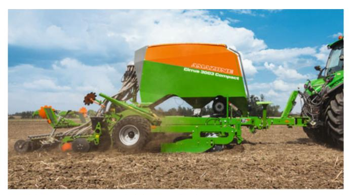
As a trailed sowing combination, the Cirrus makes higher operational speeds possible.
