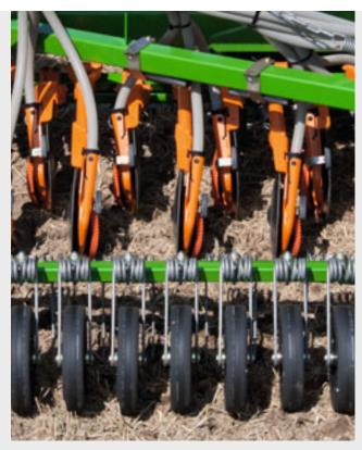
For operation in dry areas, the Citan seed drills can be equipped with a roller harrow.
