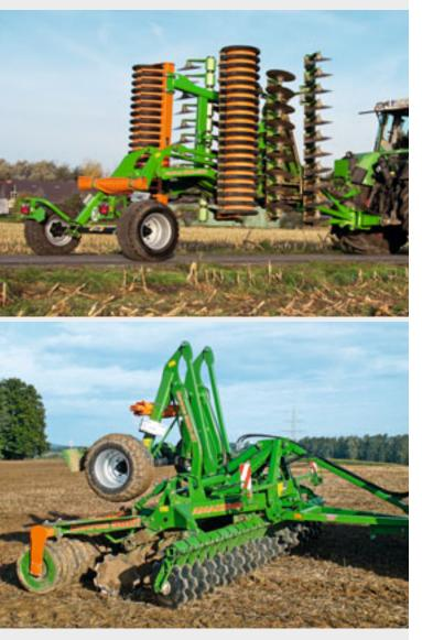
The standard equipment on the Catros-2 TS trailed machines in 4 m, 5 m and 6 m working widths includes a bogey chassis and drawbar.
