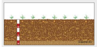
Conservation soil tillage using the compact disc harrow and cultivator with deep loosening
