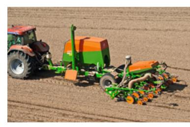
EDX 6000-T precision air seeder with 8 rows and 6 m working width.
