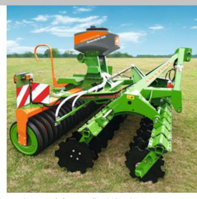
In combination with the GreenDrill seeder box, the Catros compact disc harrow can also be used for sowing fine seeds. Alternatively, the GreenDrill seeder box can also be operated with the Cenius mulch cultivator, the KG rotary cultivator or the KE rotary harrow.
