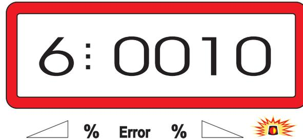
The first digit shows the chosen mode "6", the second the average forward speed in [k.p.h.] – e.g. "0010" for 10 k.p.h..
