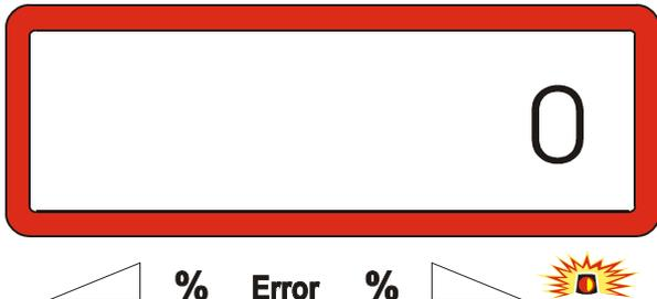
The broadcaster has been counterbalanced correctly if a "0" for 0 kg hopper content appears on the display.
