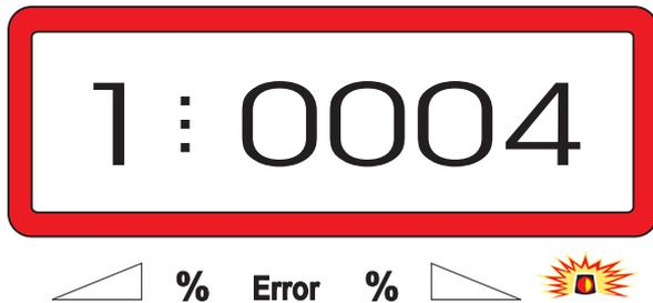
The first digit shows the chosen mode "1", the second the coding for the chosen machine type – for centrifugal broadcasters coding "0004".
