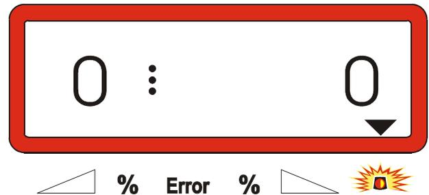
If the triangle above the warning lamp lights up, the broadcaster is not in neutral position. A constant weighing result can only be determined with the broadcaster in neutral position.
