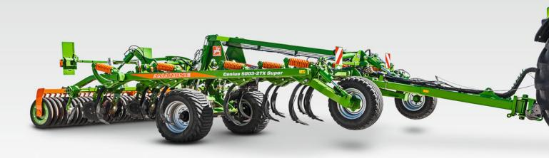
With the new TX series cultivators, AMAZONE now covers a range of working widths from 4 m to 7 m
