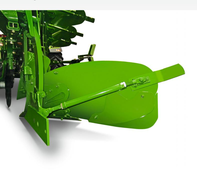
The X-Blade is a unique extension share bolted on to the mouldboard of the last plough body
