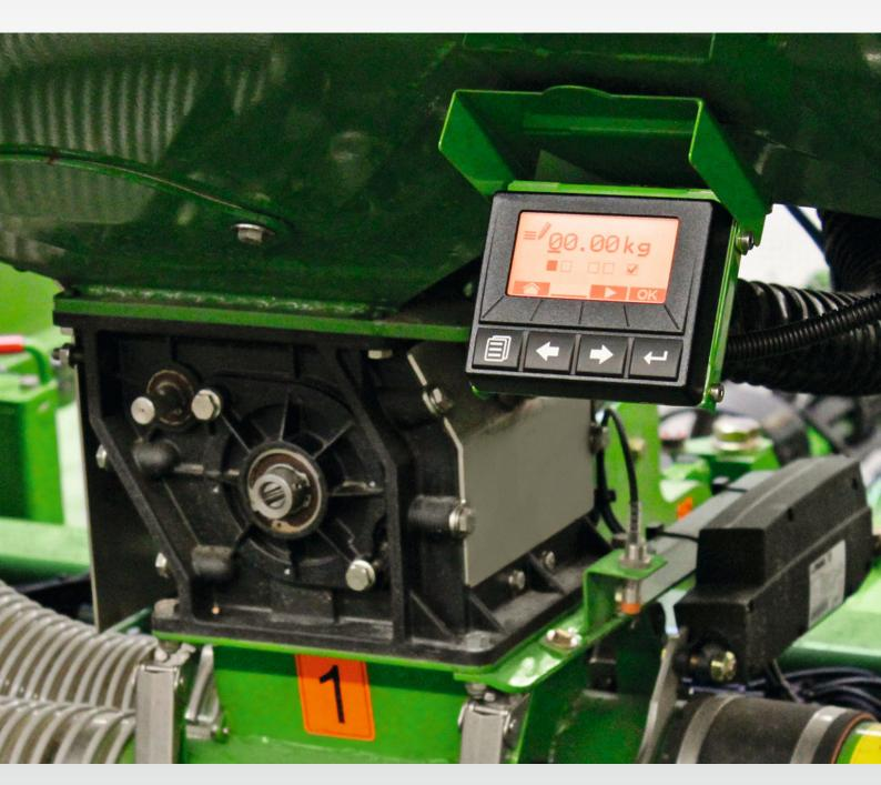
The TwinTerminal 3.0 enables the driver to carry out the calibration procedure from ground level, directly entering the data down at the machine
