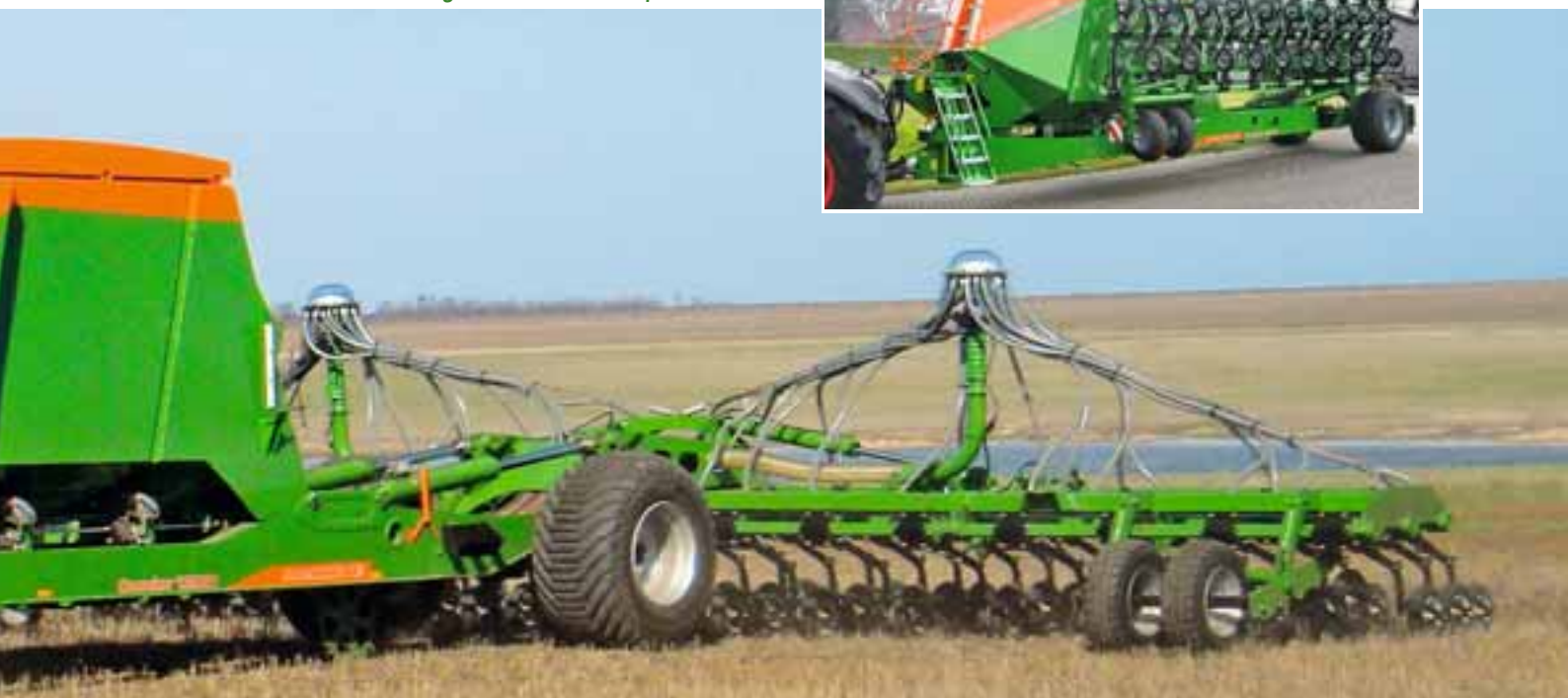
Condor 15001 in 15 m working width and a 3 m transport width
