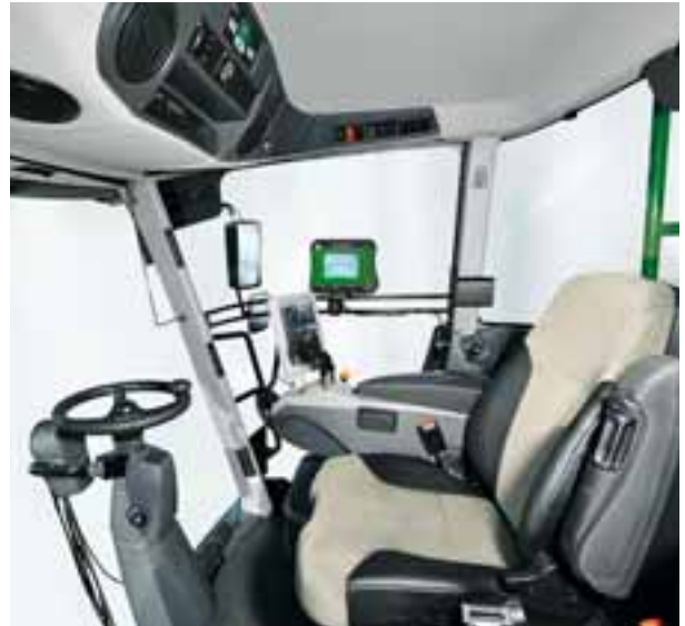
The Pantera driver's cab – with high-quality equipment, optimum all-round visibility and high operational comfort.
