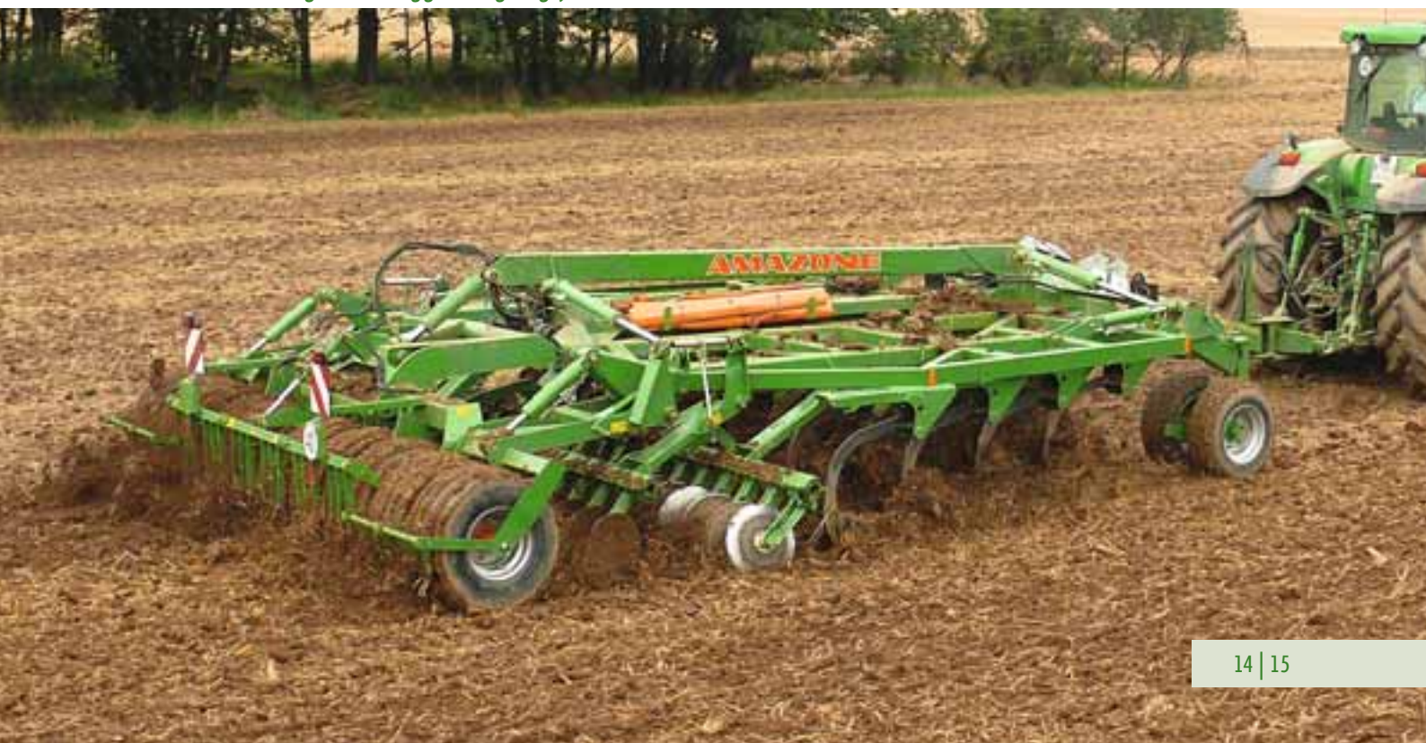
Centaur with integrated running gear, wedge ring tyre roller and 3-D tines
