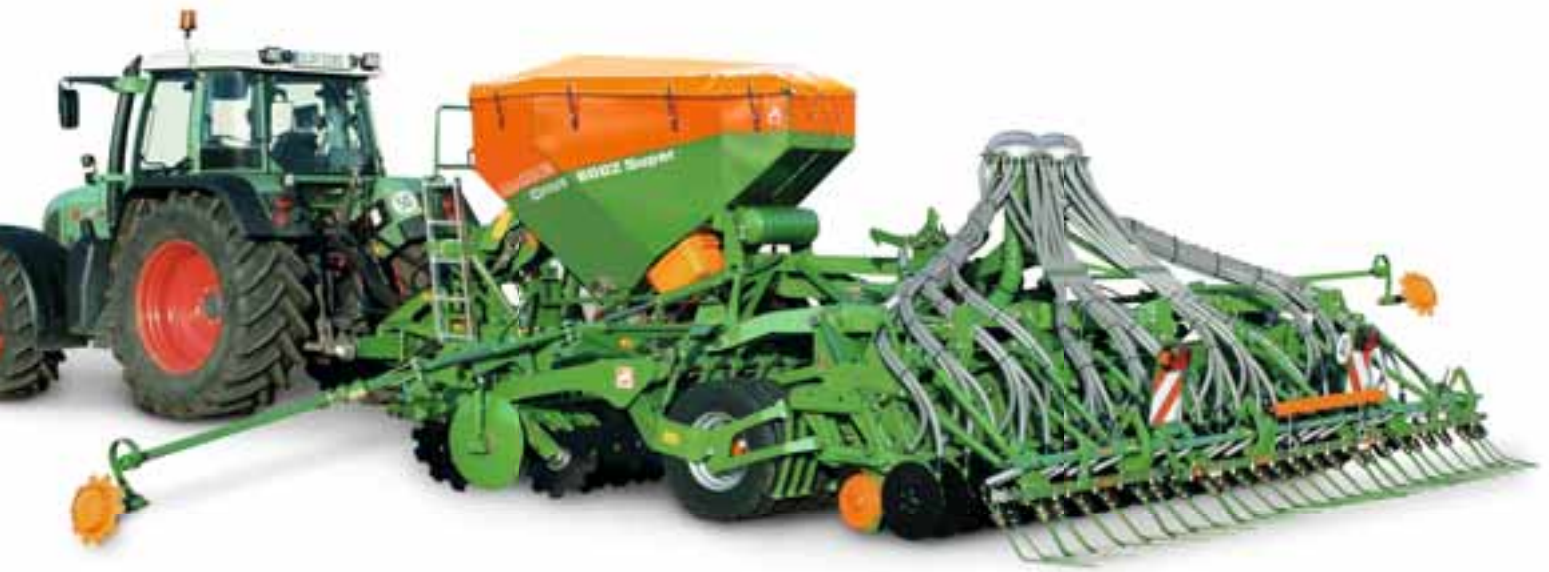
Cirrus Super with PacTeC coulters and integrated chassis
