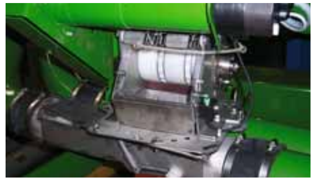
The metering cassettes in the metering unit can be easily exchanged. In this way it is possible to precisely meter all seeds and seed rates with a good longitudinal distribution even at high operational speeds.
