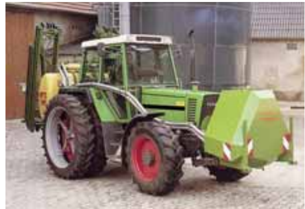
FT 802 front tank made from stainless steel
