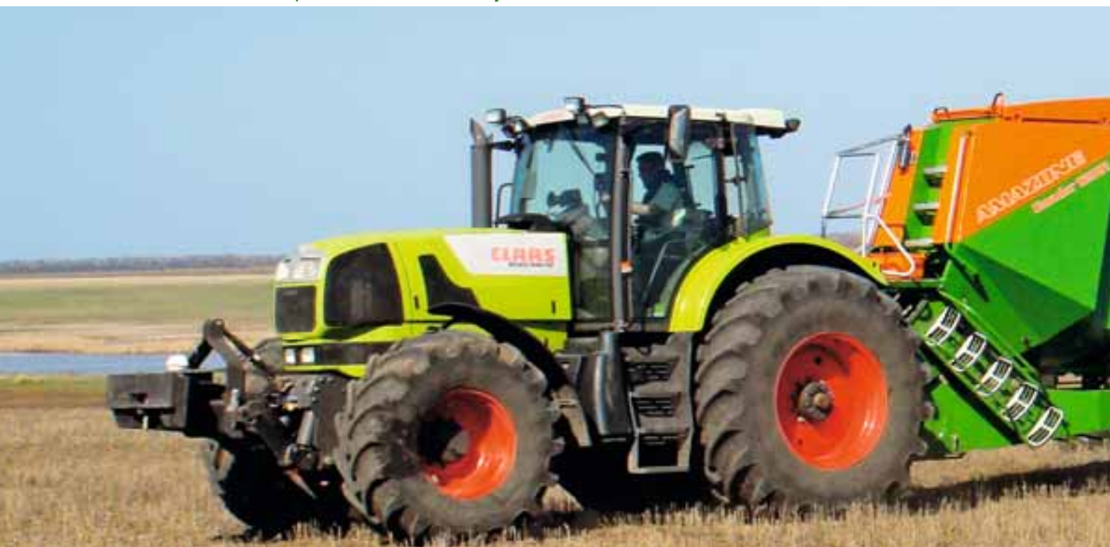
Condor 12001 with its 8,000 l pressurised tank (2/3 seed + 1/3 fertiliser)
