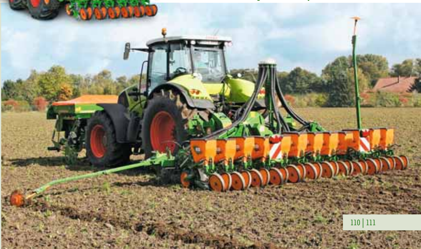
ED 602-K: narrow sowing with 12 rows and front tank
