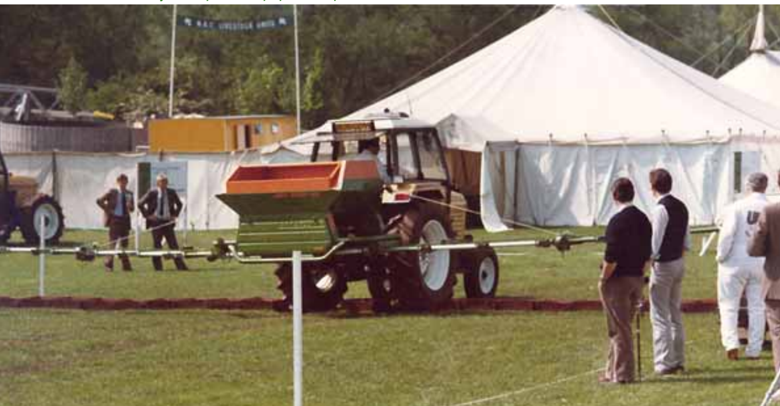
A Jet 1201 is tested for accuracy over the trays by SCAMS at Spreaders in Action in 1984.
