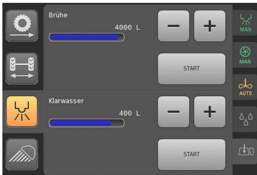
The spray liquid tank and flushing water tank can be filled at the same time and separately via the suction hose.
