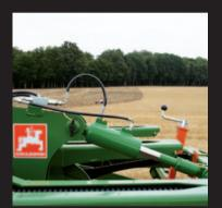
Working depth : as an option, the Cenius can be equipped with hydraulic depth adjustment.
