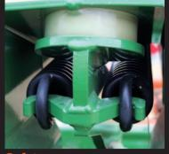
Sately : the tine is held in work by two horizontal springs and one rubber buffer. The total unit is mounted within a housing.
