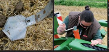
**Quick :** the share tip is fixed with a simple expansion pin which makes for an easy share change.
