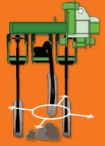
**Cenius Special** Tines with shear bolt protection, trailing spring-
